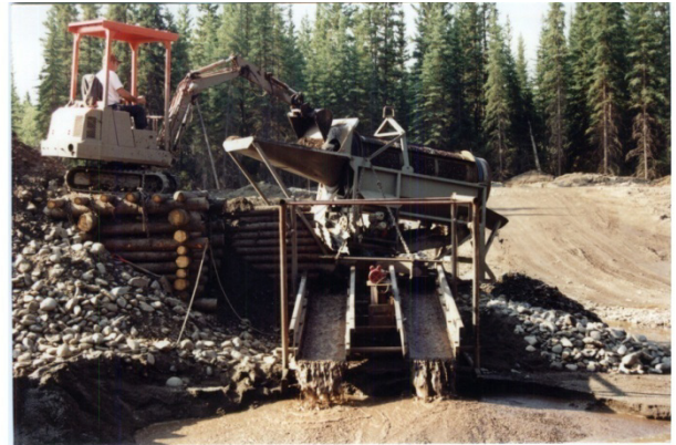
Sluicing in 1994 with oscillating boxes, 10 cubic yards per hour.
