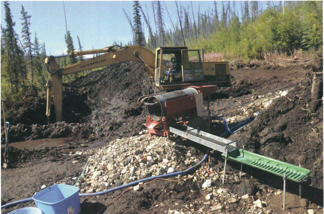
Plate 9 – The test trommel was mounted on an ATV-portable frame and had a ½ inch screen. Powered by an electrical motor with water supplied by a 1.5 inch pump, sluiced material was fed to a 6 foot aluminum sluice run with expanded metal riffles over unbacked Nomad matting, followed by 4 feet of a "Le Trap" sluice run. Gravel was fed directly to the hopper by the excavator.
