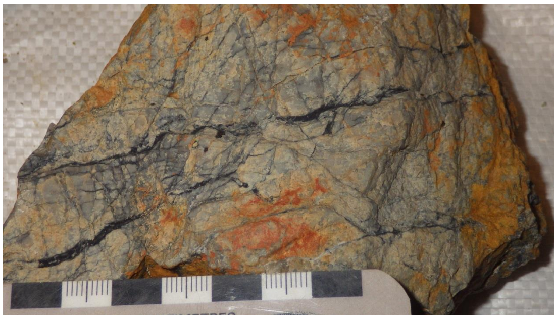
Figure 18. Sample 15NI14 altered chert with graphitic veinlets
