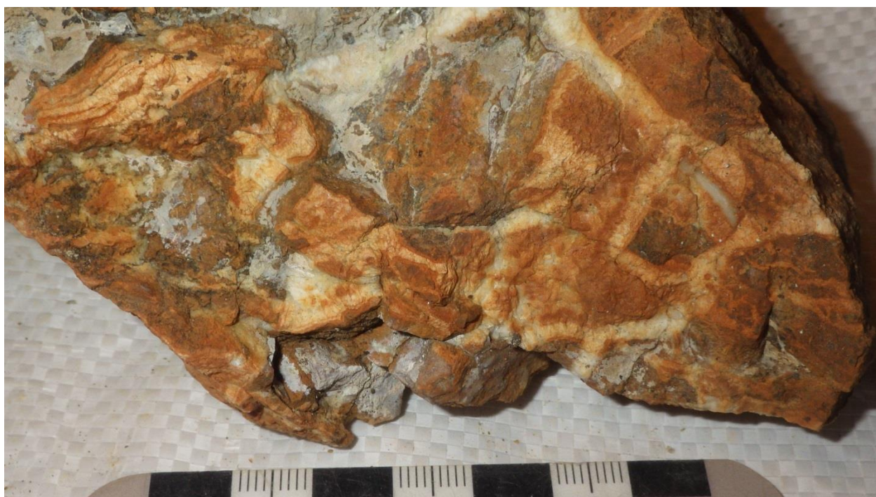
Figure 12. Listwanite alteration and quartz-calcite breccia
