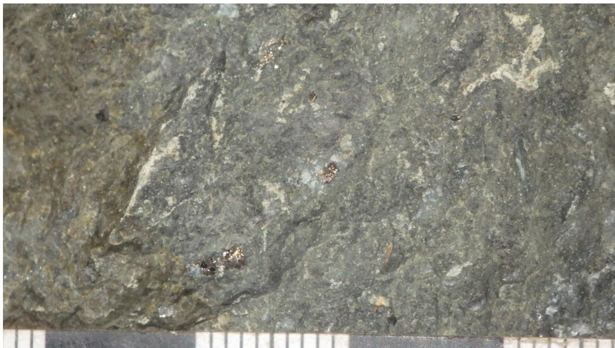
Figure 9. Commonly seen pyrrhotite blebs in altered peridotite, greenstone
