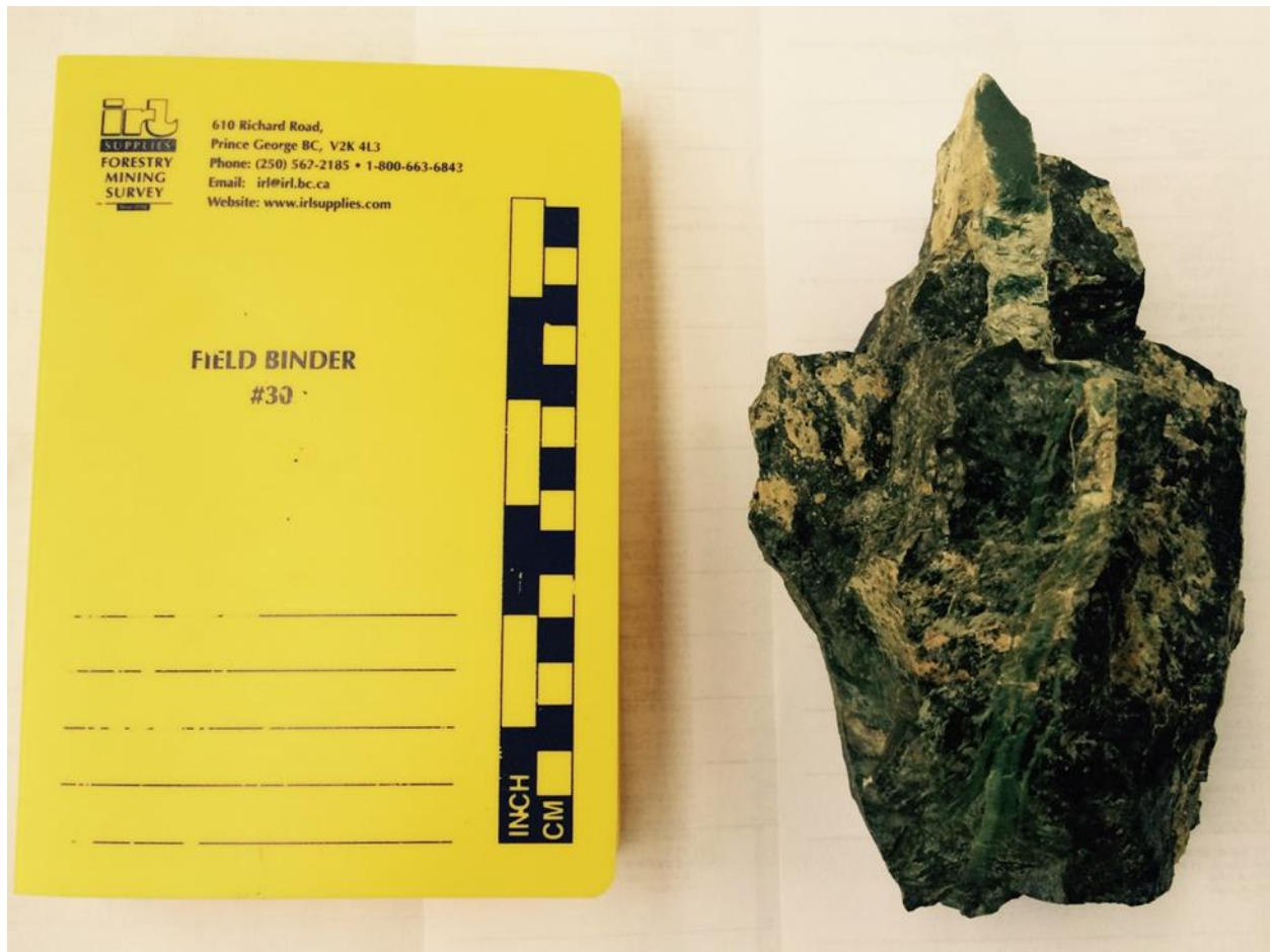
Figure 5. Sample of Jade found in 2014, asbestos veinlet transitioning into chrysotile and eventually swells and transitions to jade towards the top of the image.
