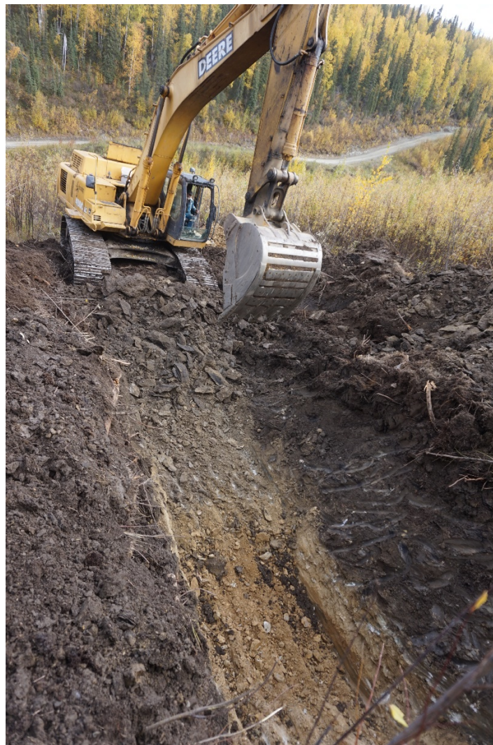
Figure 3. Discovery test pit showing gravel at the base below frozen muck. UTM coordinates: 596114 E, 7079906 N
