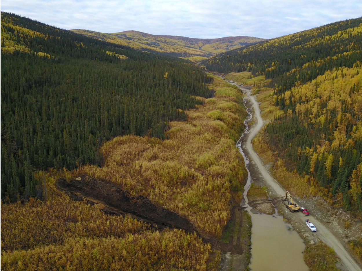
Figure 13. View looking upstream with the discovery trench in the foreground. The intermediate-level bench will be partially overlain by modern strippings of muck. A high-level bench may be present further upslope but will have thicker overburden accumulation.
