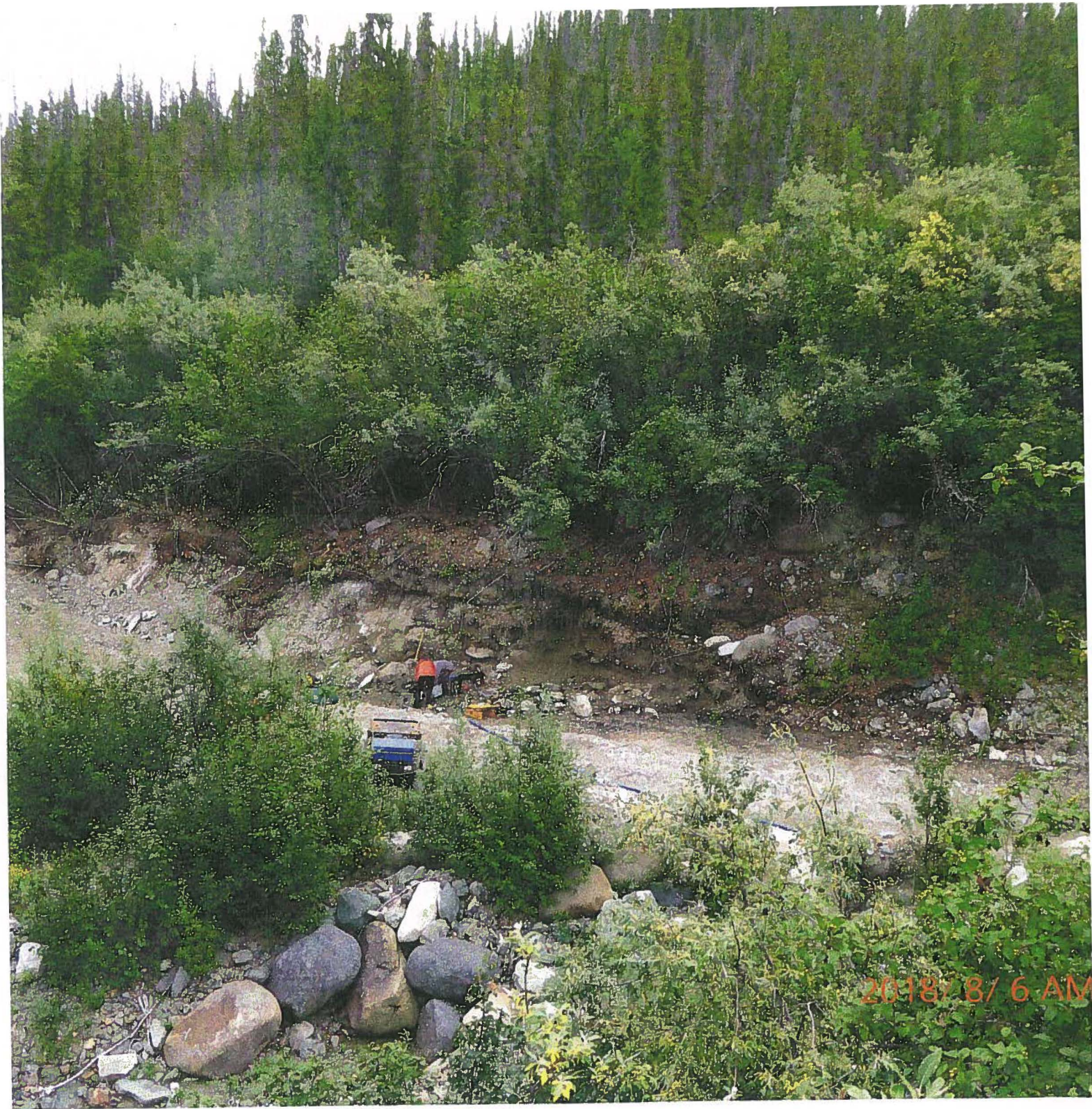
Photo 9: Looking west at the Right Limit face of Block 1 in the area of Trench 3. The foreground has been mined and is made up of low profile stacked tailings. The top of the Block is covered by alders with muskeg and stunted back spruce covering the steeper slope to the east. The faint line along the lower face of the bench, marked by the head of the backhoe is the line of sampling along the contact of the bedrock and the overlying gravels..
