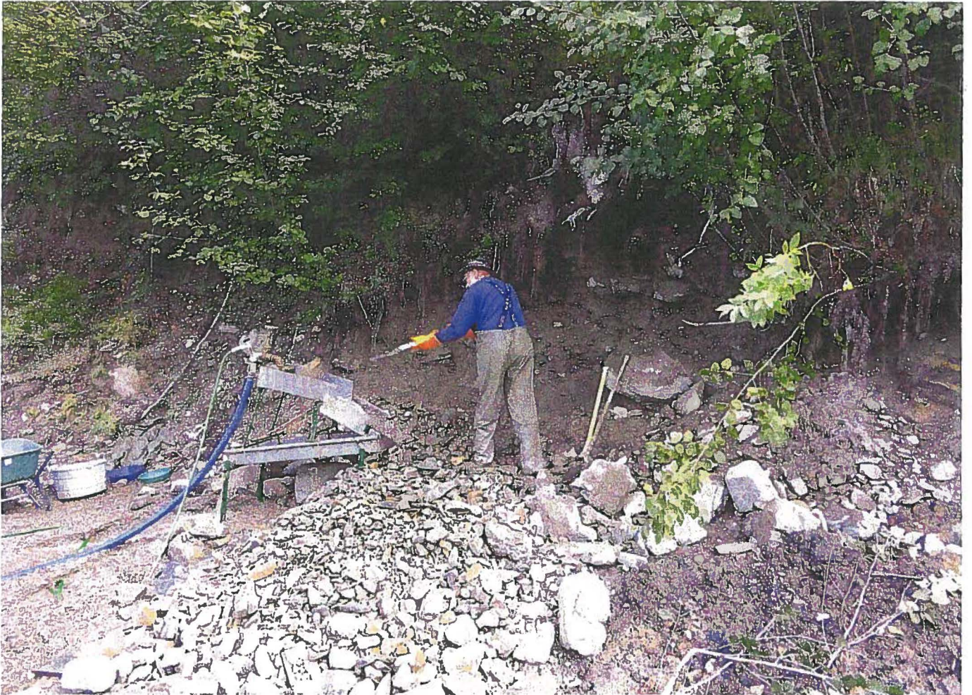
Photo 3: 2019 new sluice set up in Trench 3. Note oversize tailing pile
