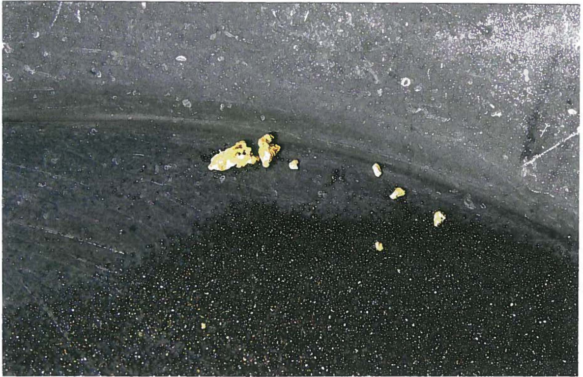
Photo 10: Sample from Left Limit trench at outlet of Lower Canyon showing course hackley gold and black heavy mineral concentrate in metal gold pan
