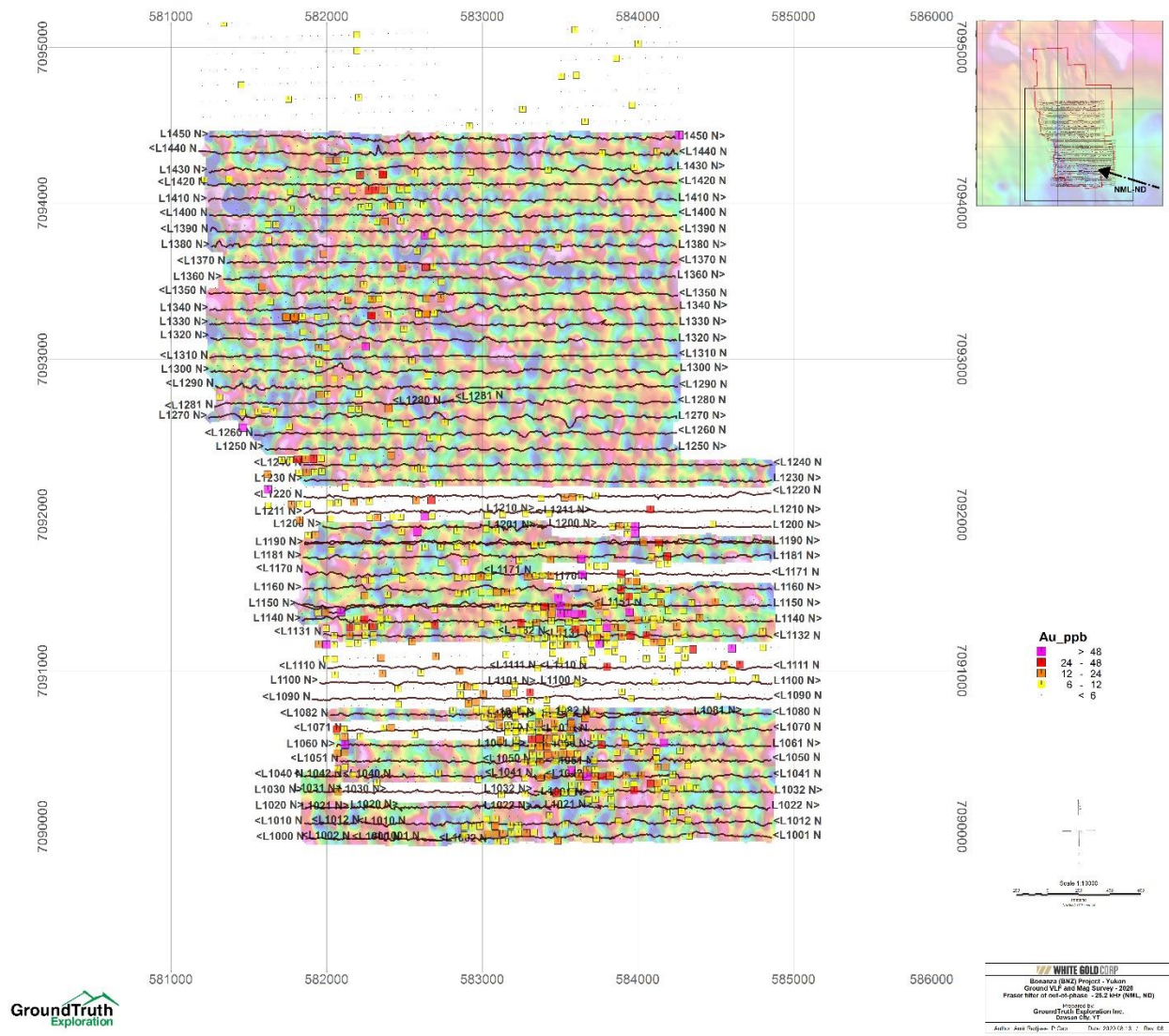
Figure 9: Ground VLF-EM survey 2020, Fraser filter of out-of-phase signal frequency 25.2 kHz NML, ND, USA.
