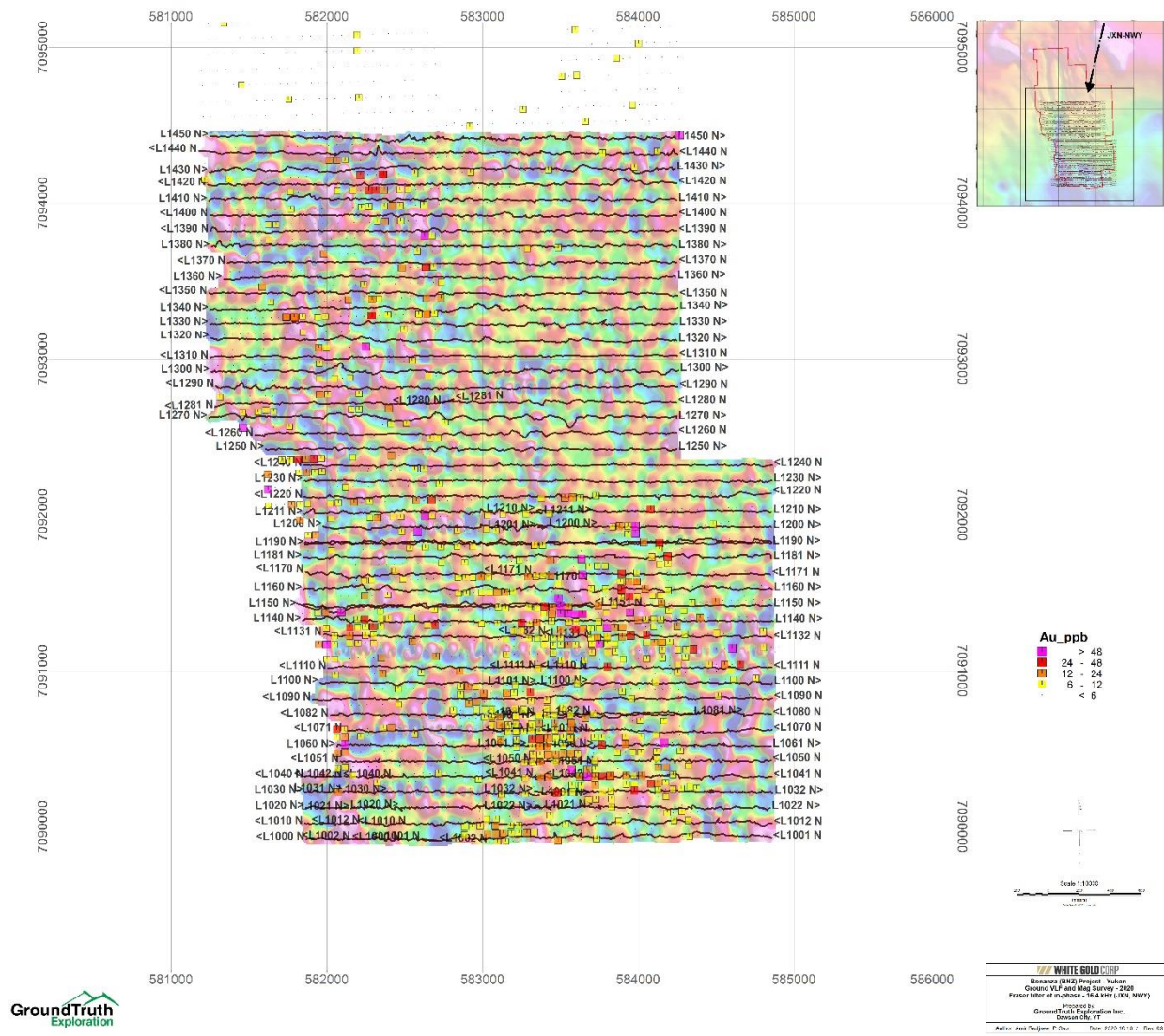
Figure 4: Ground VLF-EM survey 2020, Fraser filter of in-phase signal frequency 16.4 kHz JXN, NWY.
