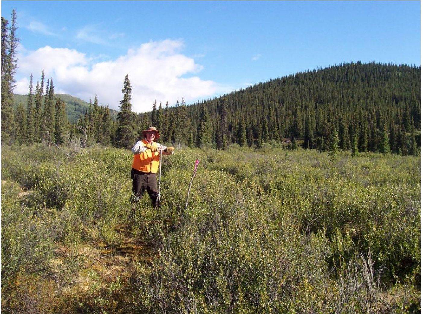
Photo 2. Looking north at W. Hood auguring through sand at surface to determine depth to underlying fluvial gravels at 1780E/3320N.
