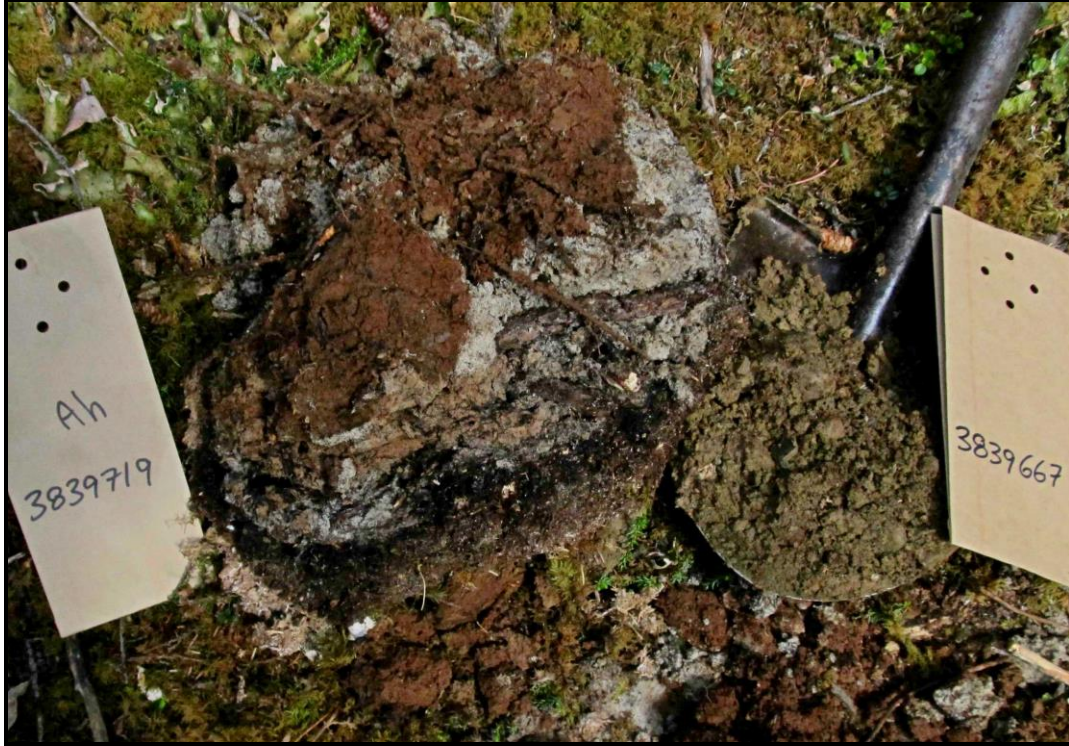
Plate 5. Inverted soil profile showing red-brown B horizon over White River ash, over Ah horizon (sample 3839719), over organic layer, with C horizon (sample 3839667) in shovel.
