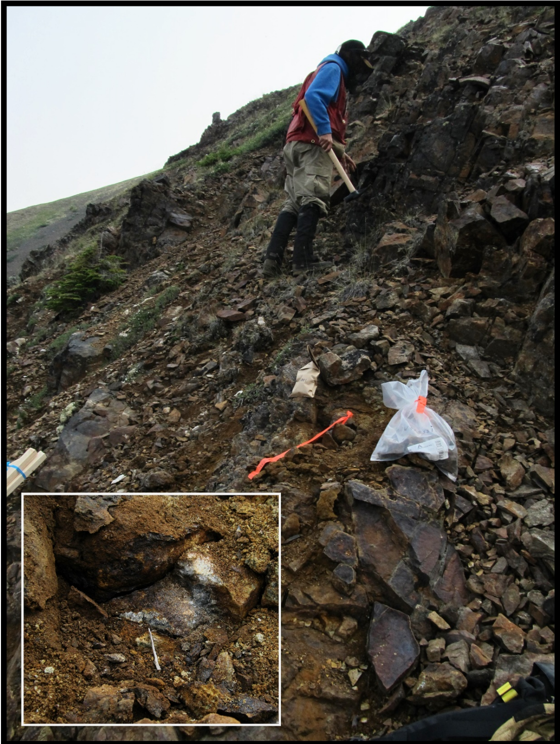
Photo 5: Main Showing area, sample W425881. Analysis returned: 0.361 g/t Au, 292 ppm Bi, 4380 ppm W from the pyrrhotite dominant sucrosic quartz-chlorite mineralization hosted in black shale.
