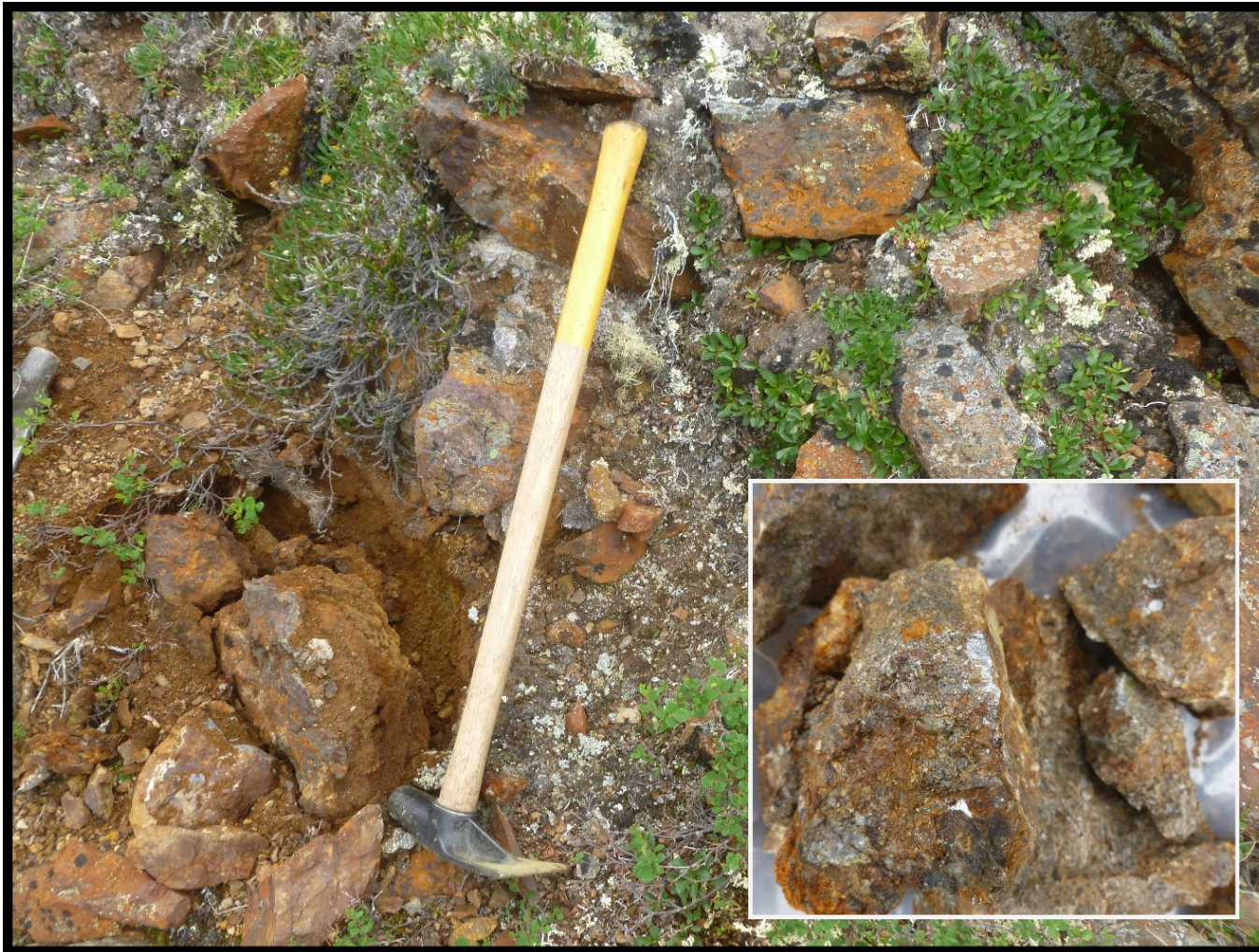
Photo 6: Copper Soil Anomaly area, rock sample W425935. Analysis returned: 0.049 g/t Au, 7.5 ppm Ag, >10,000 ppm As, 31 ppm Bi, 4.52% Ca, 595 ppm Cd, 2600 ppm Cu, 1.52% Zn. Nearby 2020 soil sample Y647774 returned: 0.032 g/t Au, 66.8 ppm Ag, >10,000 As, 18.8 ppm Bi, 141.5 ppm Cd, 1210 ppm Cu, 191 ppm Bi, 3740 ppm Zn.
