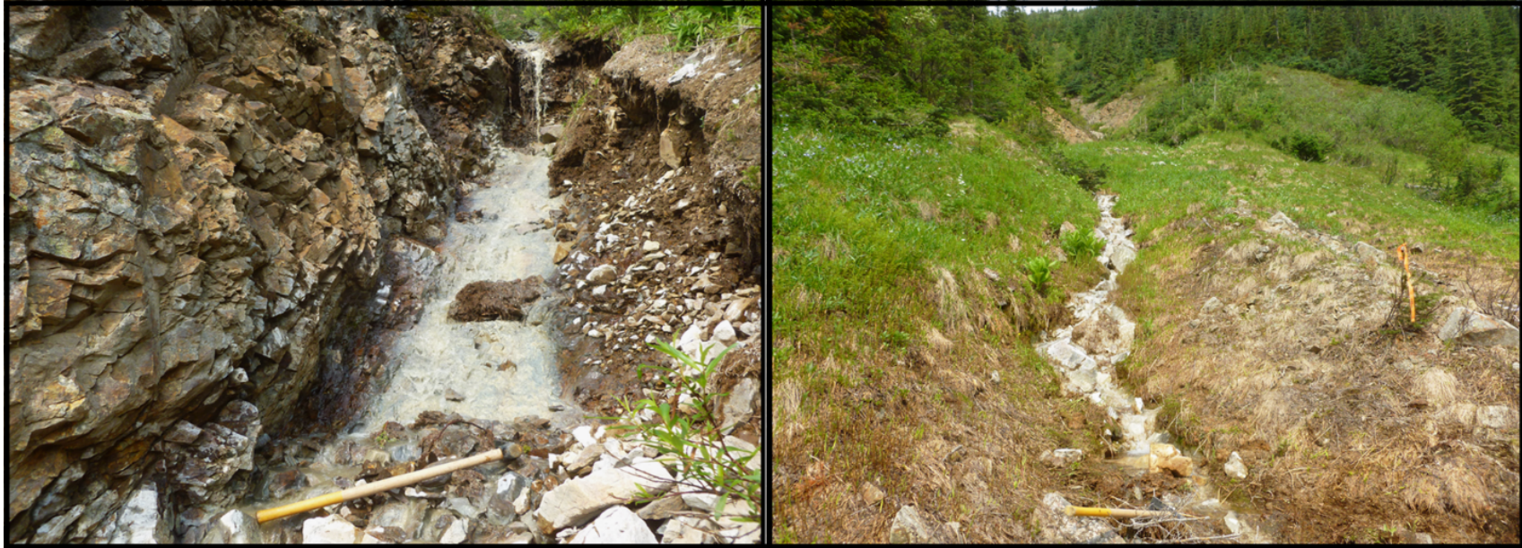
Photo 14: White stained creek (left) and silt sample M895641 (right) approximately 600 m north of the LM showing area. Analysis returned: 247 ppm As, 637 ppm Cu, 29.4 Mo, 219 ppm Zn, but negligible Au. White staining up stream is correlated with the high aluminum content (11.4%). This was also observed in the creek draining the known intrusion outcropping in the central part of the Acta claim block (where sample Y647768 returned: 2510 ppm As, 653 ppm Cu, 39.1 Mo, 77.5 ppm W, and 10.1% Al). The white staining interferes in the identification of the rocks, the “cursory traverse” failed to identify intrusive rock, but the near surface intrusion and major fault is suspected.
