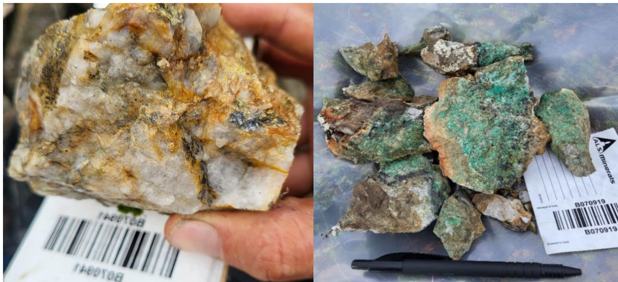
Figure 6: (Left) Sample B070941 assayed 0.816 g/t Au, 74 g/t Ag, 1340ppm Mo, and associated with 5060ppm Bi. (Right) Sample B070919 assayed 6470 ppm Cu. Both samples were taken from a 1m wide Qtz vein found within an intermediate porphyry.
