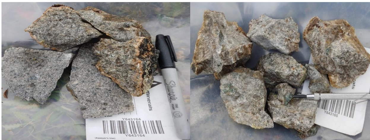
Figure 3: Granodiorite and monzonite grab samples. The monzonite sample to the right shows trace chalcopyrite, malachite, magnetite, and pyrite. Assayed 0.022 ppm Au, 3.1 ppm Ag, 211 ppm Cu, 673 ppm Pb, 907 ppm Zn. Sample Y643165.
