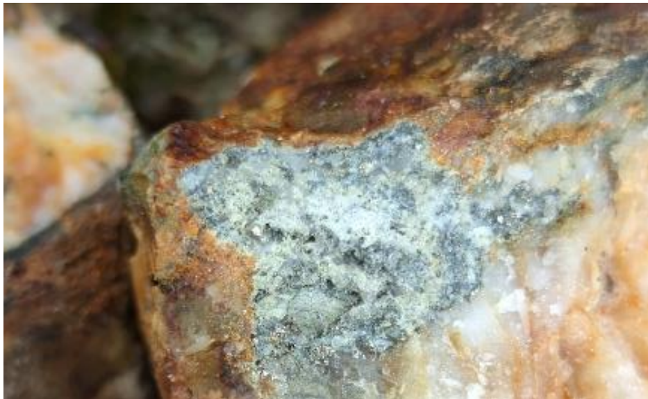
Figure 33 – SRC286212 showing fine grained arsenopyrite along vein margin. Field of view is approximately 4 cm.
