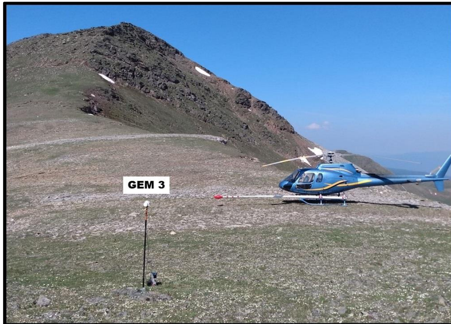
Figure 17: GEM 3 magnetic base station.
