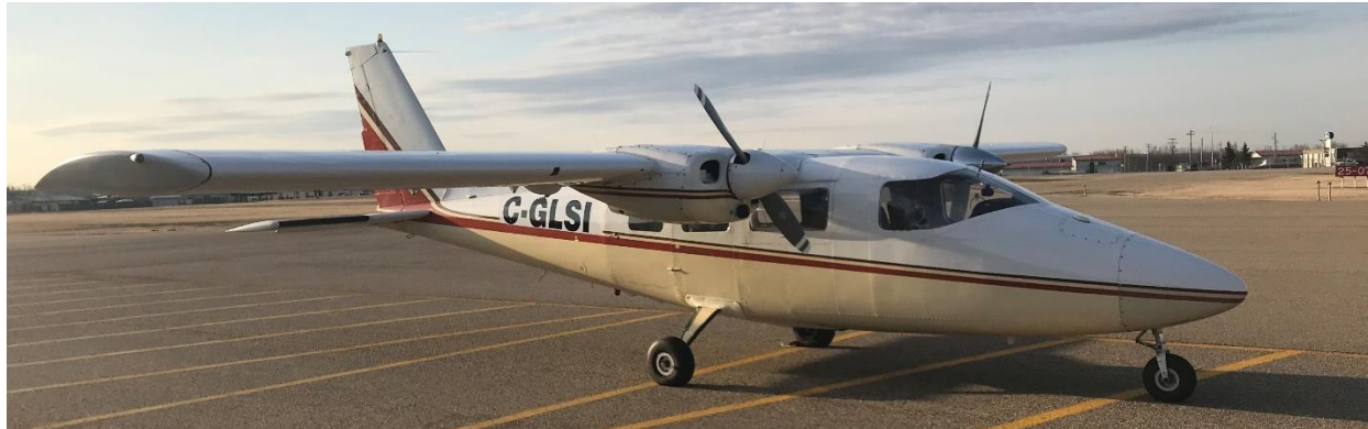
Figure 1: P68 with MATRIX LiDAR System
