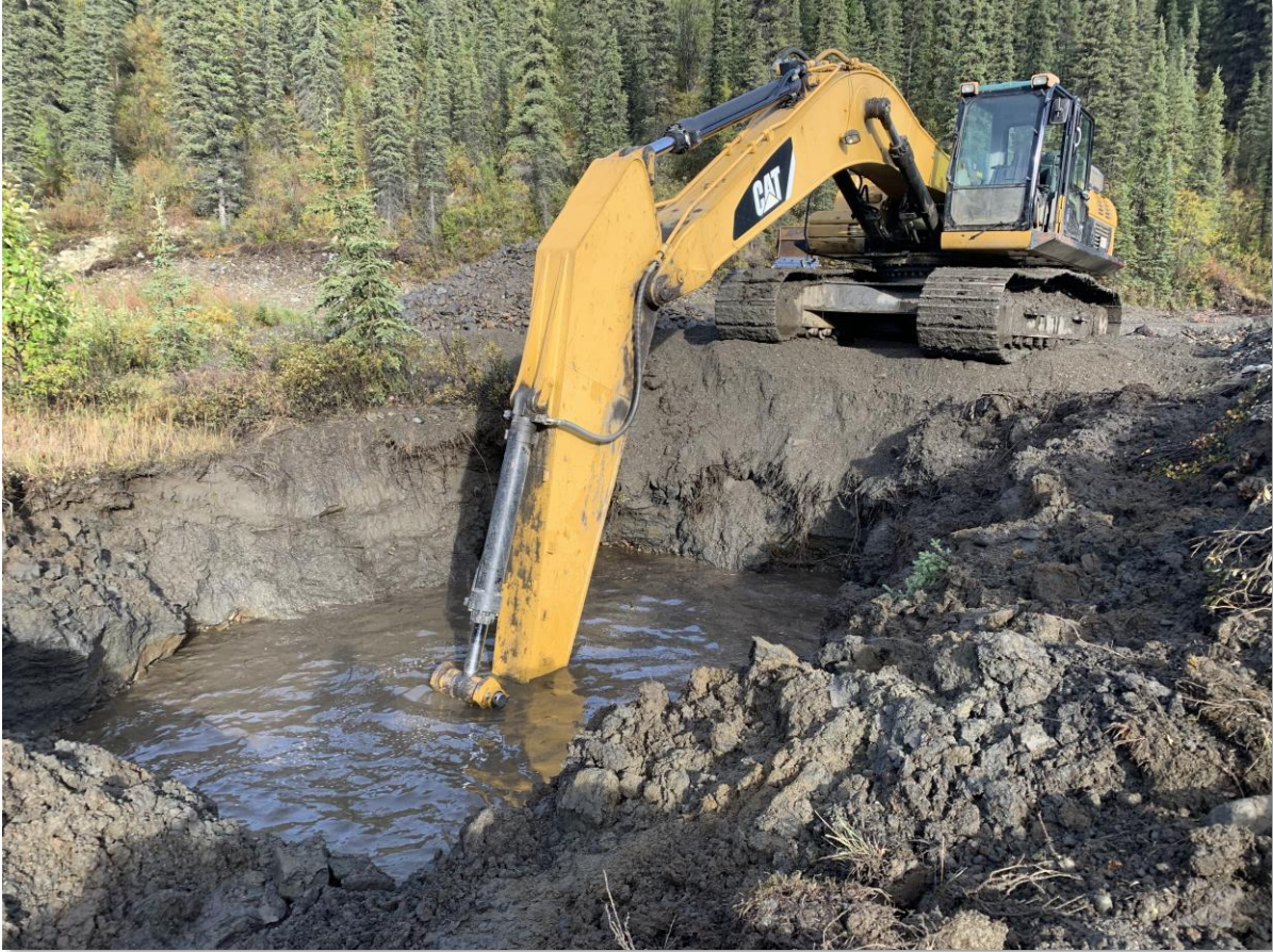
Figure 10 - The surface gravels were tested with a CAT 330DL excavator at depths from 0 to 12 feet. The first five bulk samples (22-1 to 22-5) were from creek gravels located on the Bruces 1 claim.
