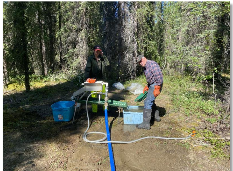
Figure 8 - Drill samples were processed using a LeTrap sluicibox with a wet hopper fed with a 2-inch pump. Concentrates were hand-panned.
