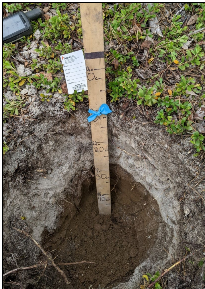
Figure 7-3: Example of a sample with a thick layer of volcanic ash. In these conditions the sample would be collected immediately below the base of the ash layer.
