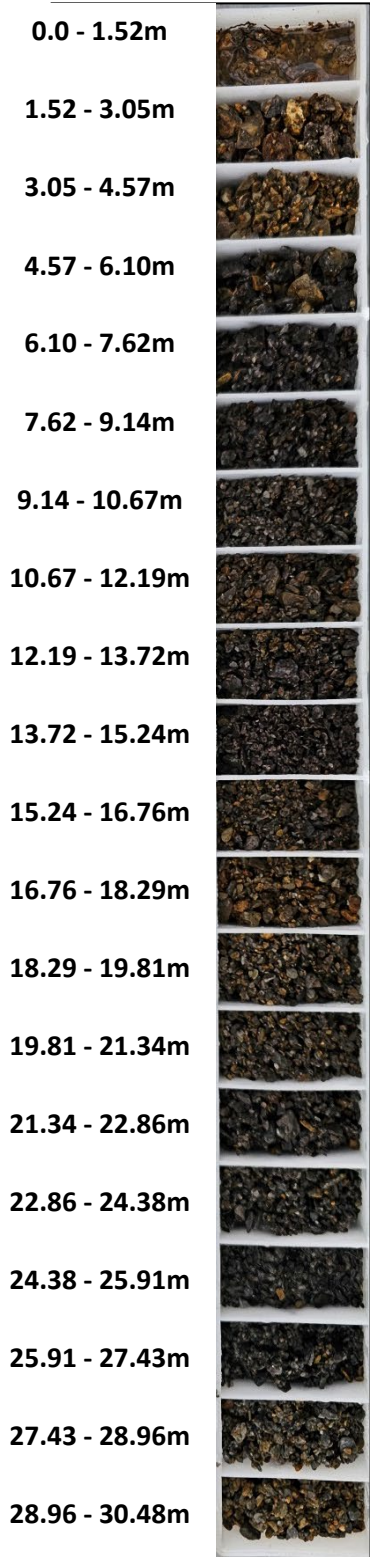
Photo 8. WLFTRS23RAB002 Chips showing mineralized and oxidized intervals (0.0-30.5m).
