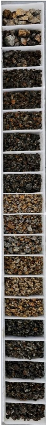
Photo 5. RAB Chip tray for WLFTRS23RAB0010.0-30.5m with oxidized andesite interval (45-75ft).
