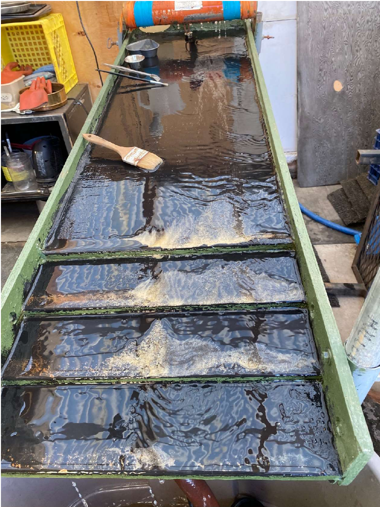
PHOTO #21 Miller table in operation and gold recovery equipment
