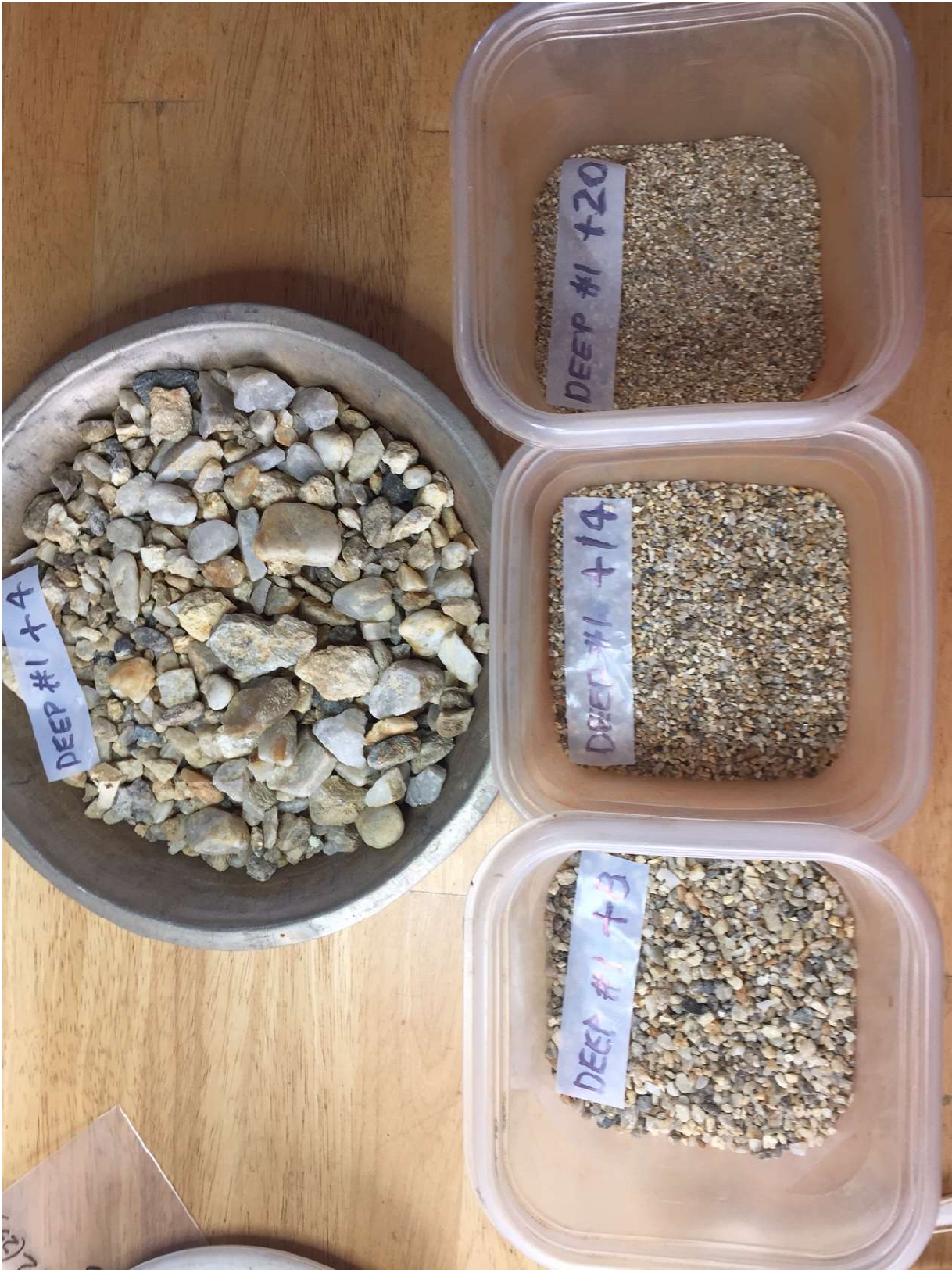
PHOTO #20 Sieved coarse fractions of longtom concentrate from bulk sample tub #1
