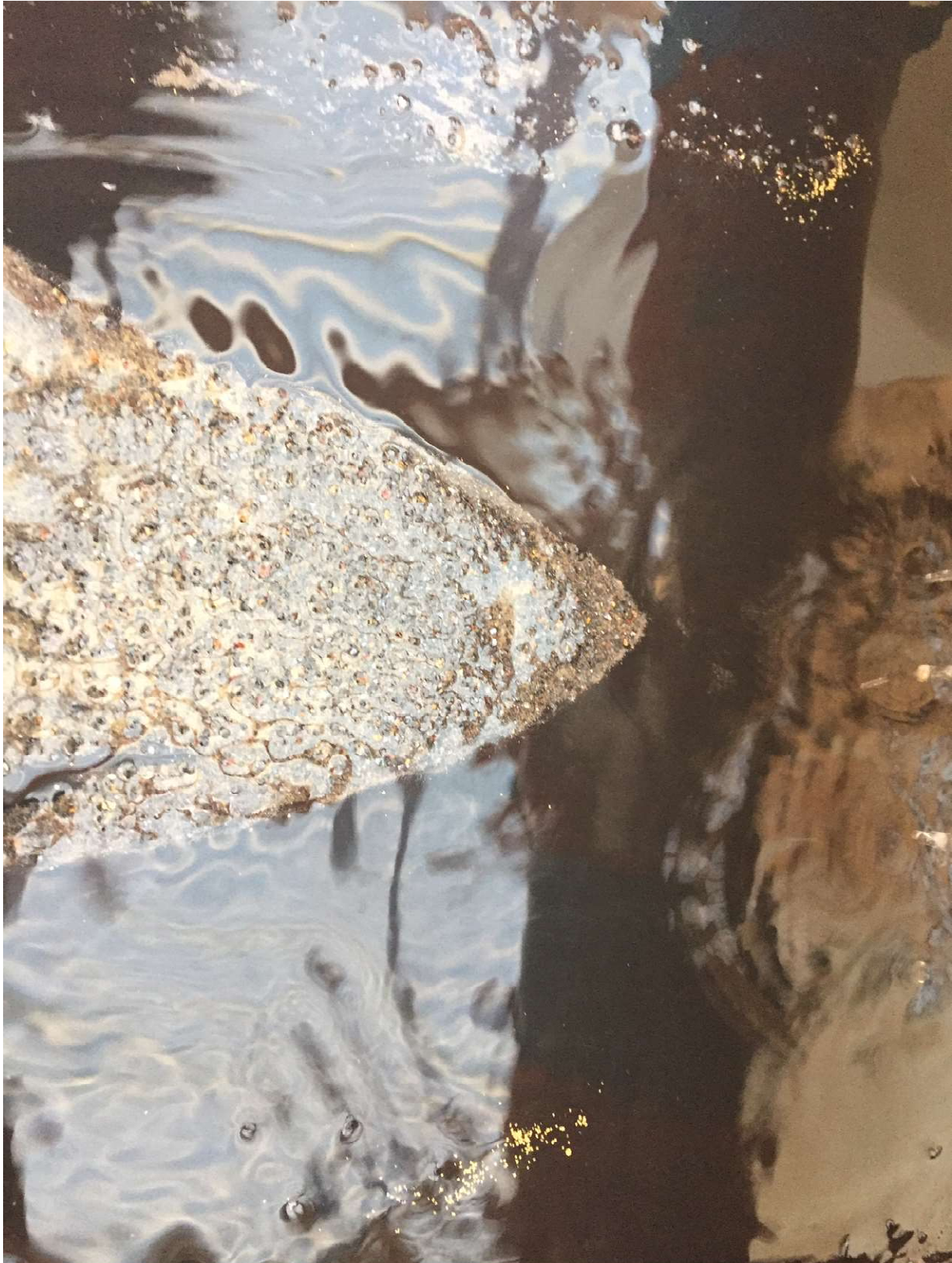
PHOTO #24 Fresh portion of sample just placed in center of miller table – clusters of gold particles separated from previous portions of sample on both sides.
