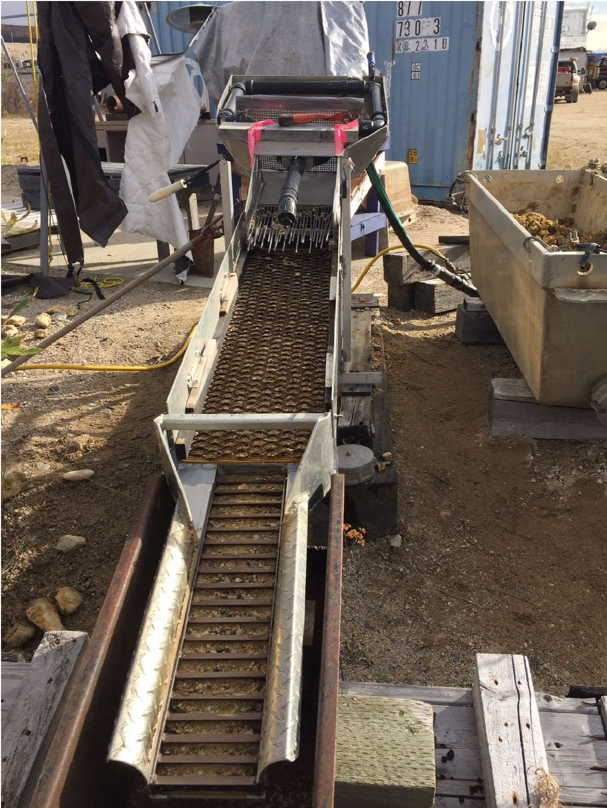
PHOTO #15 Longtom used in 2023 Bulk Sampling Top right is Deep bulk sample tub-#2
