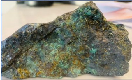
Figure 9.0 Grab sample. Rocks are heavy, magnetic and black with deep green/blue and have visible sulphide inclusions.
