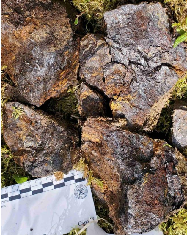
Plate 6. Pit 4 (2023) Sample 26151. Massive goethite with 1012ppm Cu, 981ppm Zn, 4.8ppm Ag, 3289ppm As, 38% Fe.
