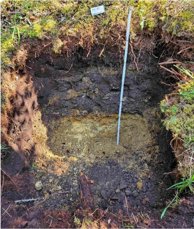
Plate 8. Pit 11. Iron rich subcrop beneath buried organic layer.
