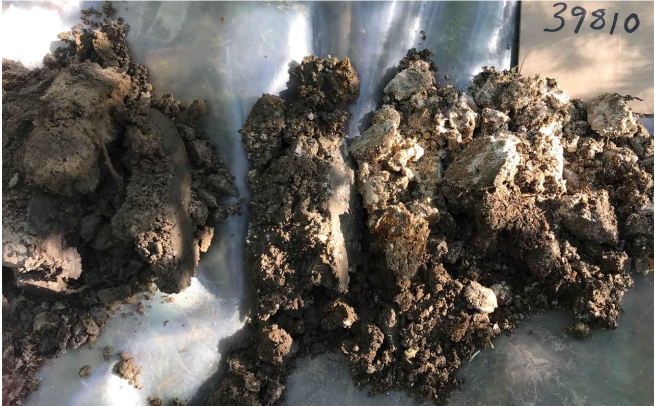
Plate 4. Soil sample #39810. High Cu, Zn, Ag, As, Ca
