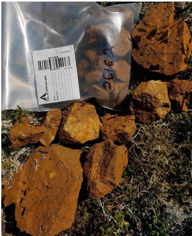
Plate 7. Pit 10 Rocks. Up to 1968ppm Cu, 4078ppm Pb, 2233ppm Zn, 20% Fe, 2160ppm As.
