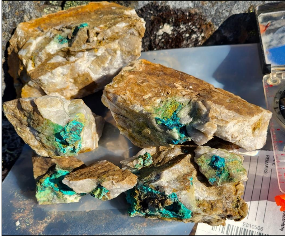
Figure 12: Sample E810505 assayed 3730 ppm Cu, 7.1 ppm Ag, 319 ppm Pb.
