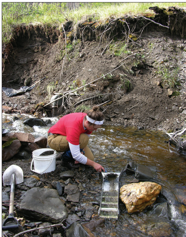
Figure 6-8. Using a portable sluice box to concentrate heavy minerals on a tributary to Grayling Creek (sluice sample). Alluvium was first pre-screened with a 4 mesh screen. The -4 mesh sediment is a manageable size fraction for the small sluice, and pre-screening allows fine sediment to be decanted out-of-stream eliminating suspended effluent into the creek.
