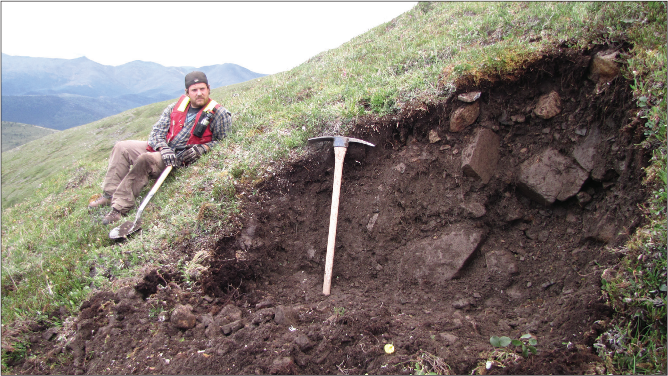
Figure 4-12. A soil pit within a solifluction lobe north of Mount Pattison (10JB054). The lobe contains abundant coarse rock fragments mixed with organics and minor silt.
