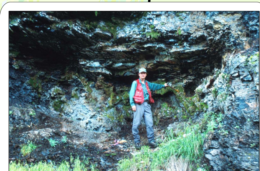
Stewart Harris (Equity Engineering) points to the massive stromatolite sulphide horizons on Blackstone Resources' Taiga property hosted in Earm Group black shales. Samples from this unit returned values up to 5.21% Ni and 904 ppb combined Au+PGE.
