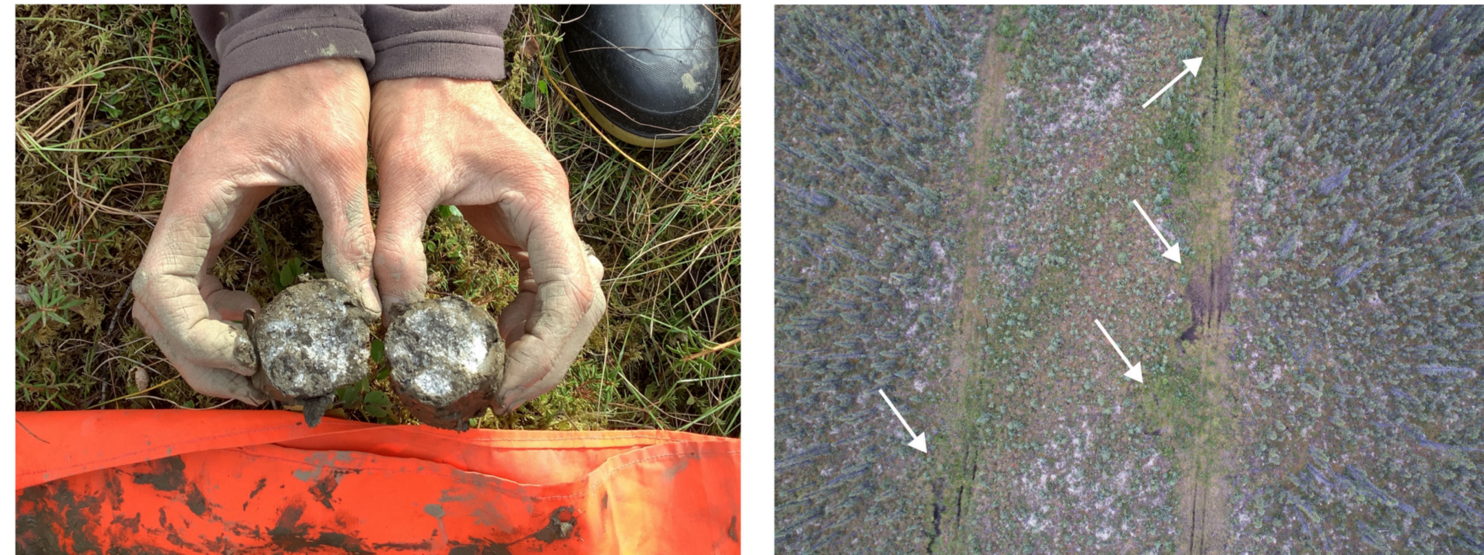
Segregated ice found in the upper 2 m of Y05, BeaverCreek, BH3 drill core. Ground ice is common within the thin loess overlying glaciofluvial outwash and within the fine-grained overbank sediments overlying the modern floodplain and fluvial terraces. Thermokarst subsidence is common along ATV trails in the map area. The compaction and disturbance of surface organics in this location reduced ground insulation and caused ice-rich permafrost to thaw resulting in ground subsidence.
