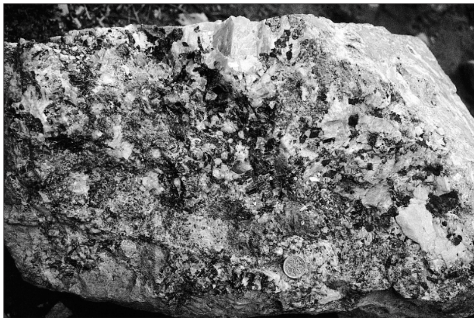
Figure 29. Chalcopyrite-bearing skarn mineralization from the Hat claims located in the Whitehorse Copper Belt.
