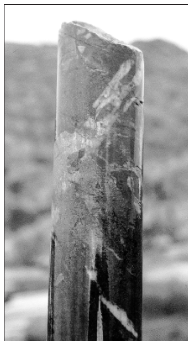
Figure 16. Bright red hematitic chert (grey in this photo) at the upper contact of a massive sulphide intersection (black) on Expatriate Resources' Ice Property in the Finlayson Lake area.
