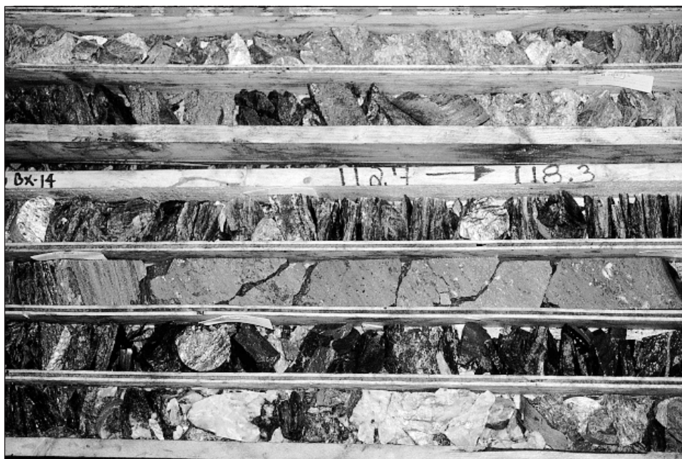
Figure 14. Massive sulphides from the Sable zone intersected in Hole WV97-106 at the Wolverine Project. This interval assayed 2.26 g/t Au, 183 g/t Ag, 0.65% Cu, 0.62% Pb and 15.70% Zn over 0.6 metres.
