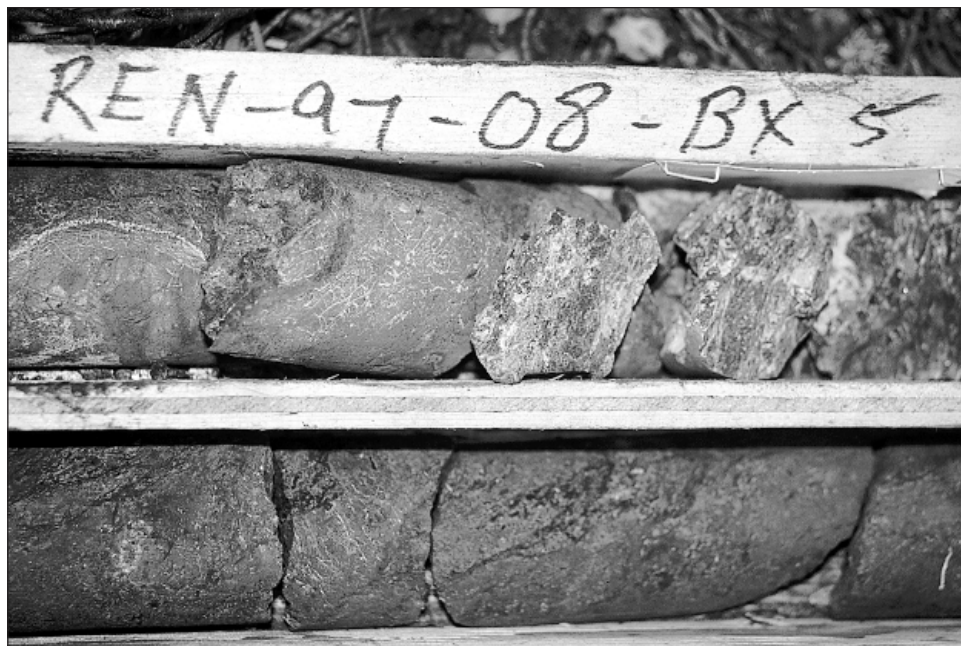
Figure 26. Drill core from Hole REN 97-08 at the Taiga property which demonstrates the subtle character of nickel-zinc mineralization. This hole returned a 5.3 metre intersection grading 1.42% nickel and 0.70% zinc.
