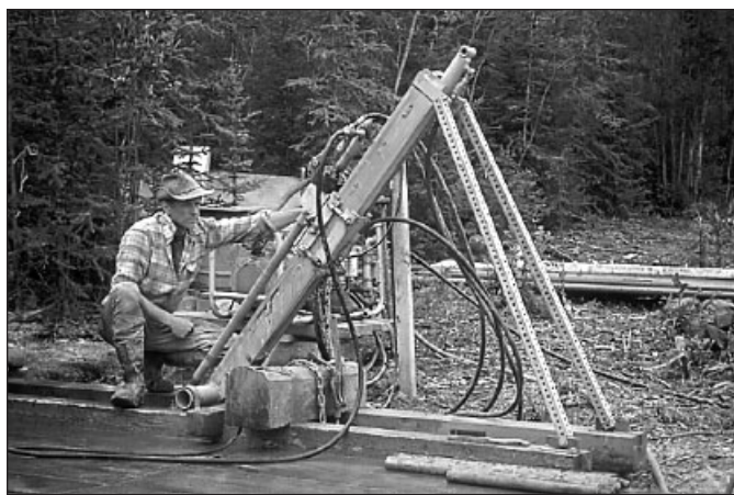
Figure 5. Al Carlos drilling on anomaly E near the Grew Creek deposit. Al and his two sons spent this past summer drilling 263 m in five holes on two properties. Photo by Ken Galambos.
