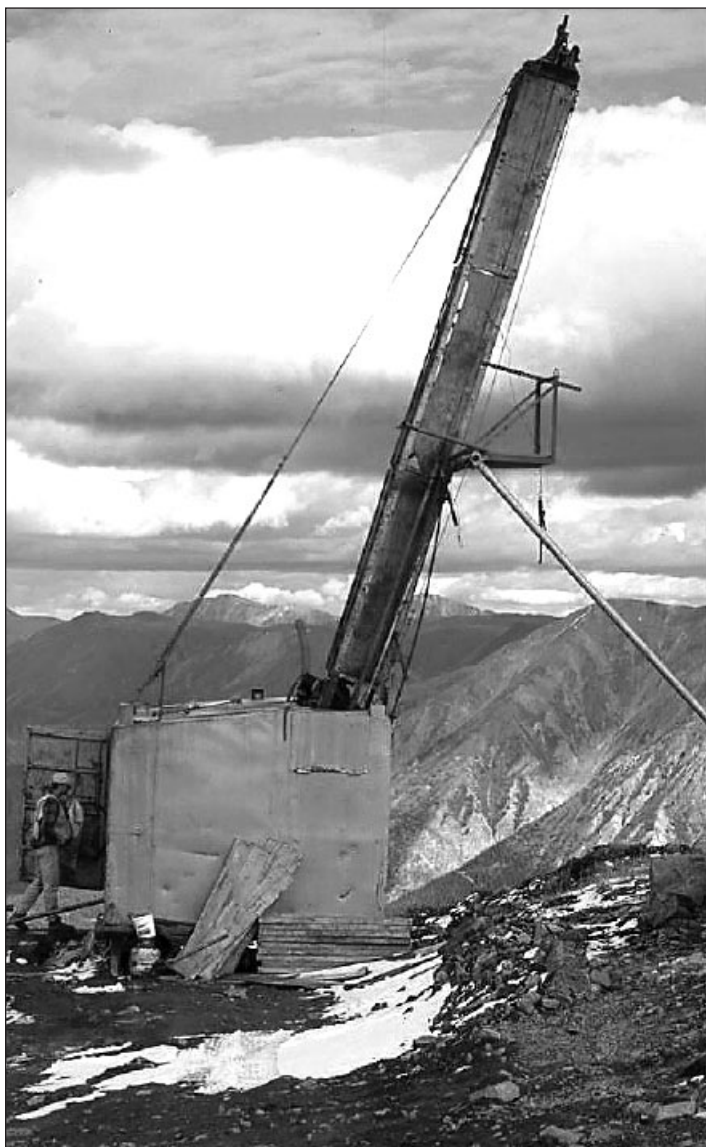
Figure 19. Diamond drill rig on the Skukum Creek property of Tagish Lake Gold Corporation.
