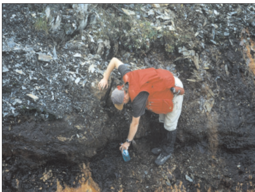
Figure 10. Water sampling of a rusty seep at the contact of black shale and overlying sericite schist. Mapping at this locality by Manson Creek Resources outlined similar stratigraphy to that hosting the Marg deposit 50 km to the east.
