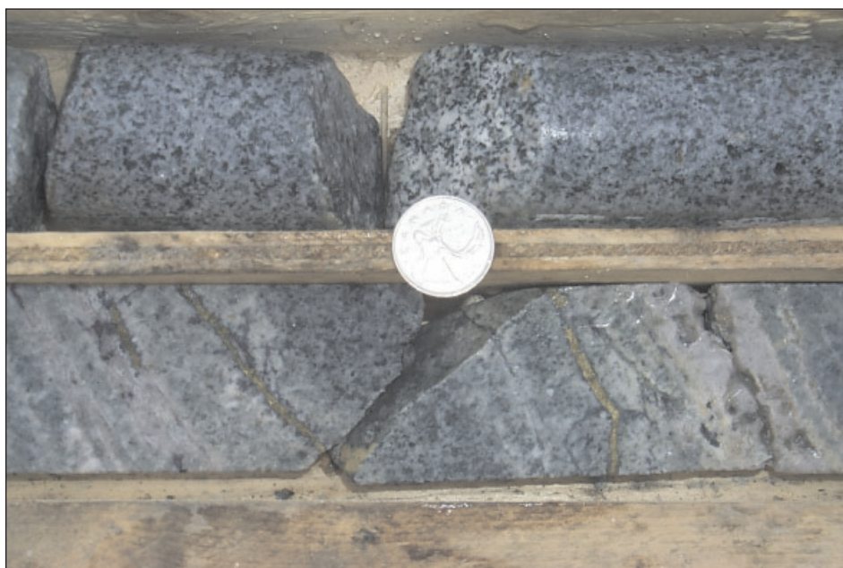
Figure 12. Sheeted chalcopyrite and quartz-calcite veining hosted in granodiorite. The drill hole targeted an IP chargeability anomaly on the Hat claims in the Whitehorse Copper Belt.
