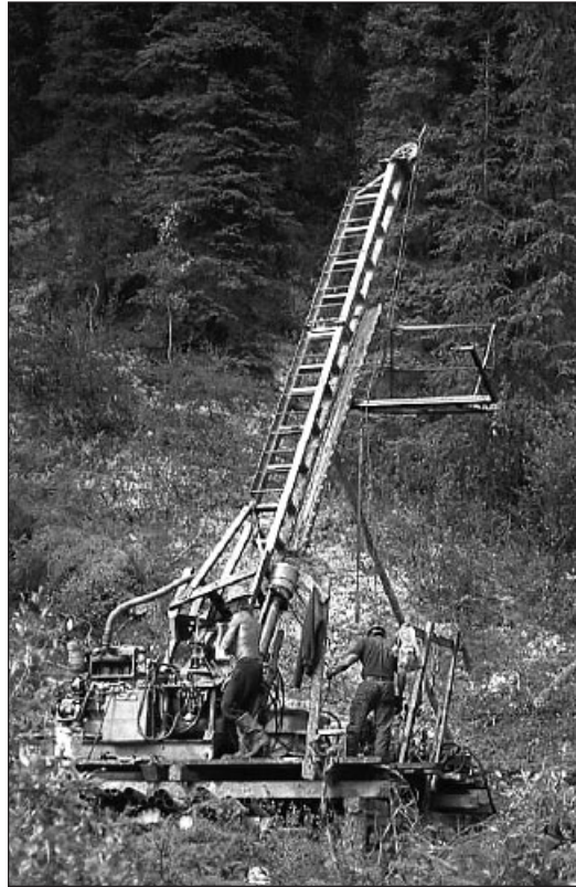
Figure 11. Noranda Exploration conducted helicopter-supported diamond drilling on the Andrew claims.
