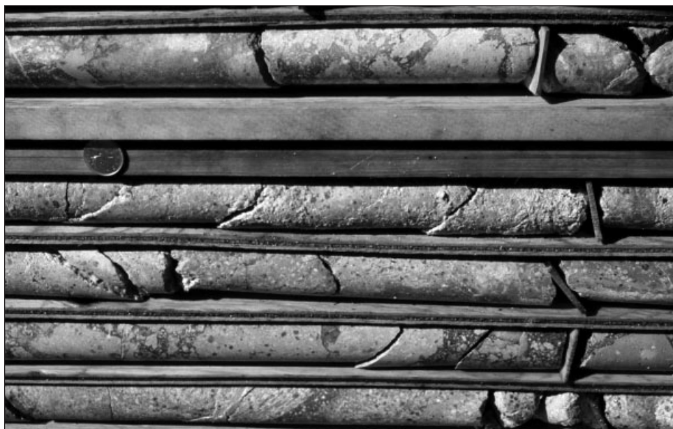
Figure 20. Hydrothermal breccia intersected in drilling on the Grew Creek property of Whitehorse prospector, Al Carlos. Quarter for scale.
