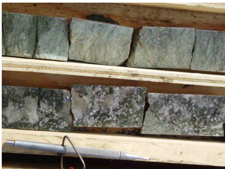
Figure 9. Chalcopyrite mineralized skarn in Mike Lake property core. Photo by Dynamite Resources.
