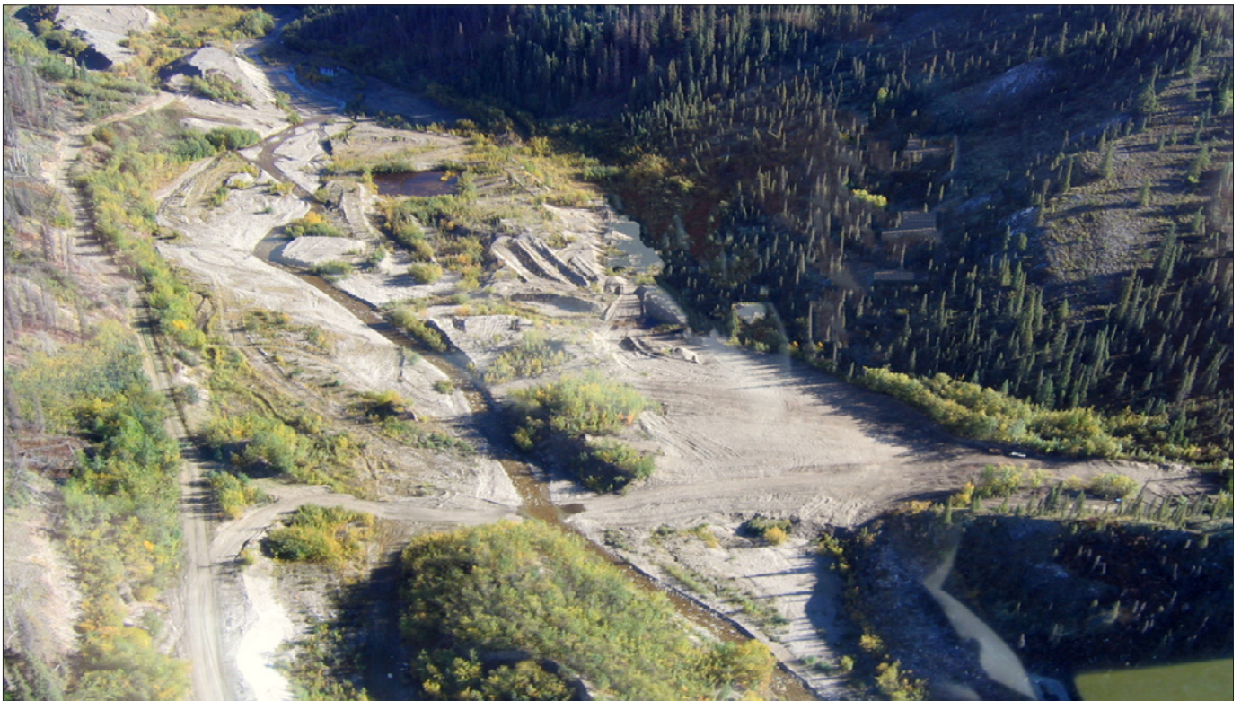
Figure 3. This is one of the sites where No Name Resources Inc. has removed the abandoned debris remaining from many years of placer operations. The site has been resloped and contoured in preparation for natural revegetation.
