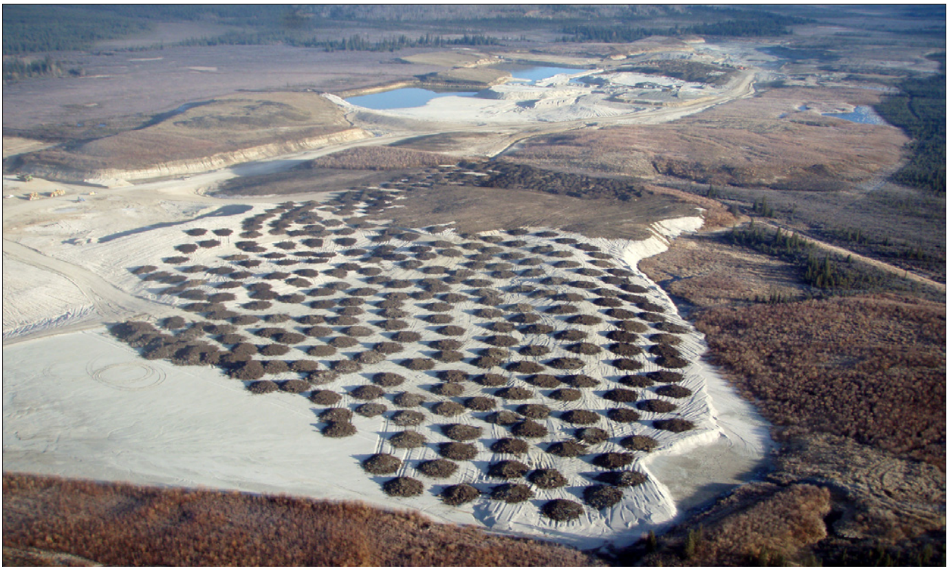
Figure 4. Ross Mining Ltd. have dumped topsoil for spreading on this sloped and contoured previously mined site.
