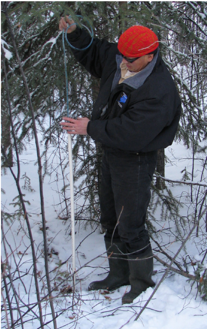
Figure 3. Typical frost tube apparatus. At weekly intervals, students briefly remove the clear tube from the white PVC casing. The depth of freezing in the active layer is indicated by the lowest depth of frozen water in the clear tube.
