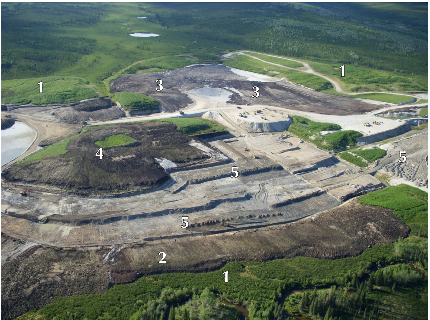
Figure 3. Placer mining continues at the Ross Mining operation next to reclaimed areas. Numbers 1 to 5 represent areas that have been reclaimed or are in the process of being reclaimed. Number 1 is the oldest and number 5 is the youngest.
