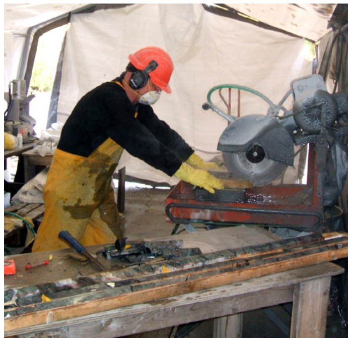
Figure 22. Technician Serge Bellemeure cutting core at the Jennings tungsten project. Photo courtesy of Agnico-Eagle Mines Ltd.
