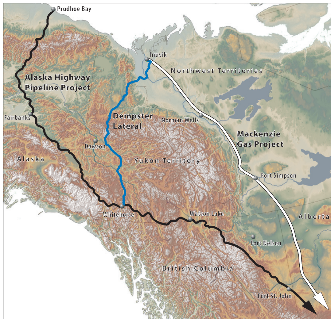
Figure 3. Northern natural gas pipeline options.
