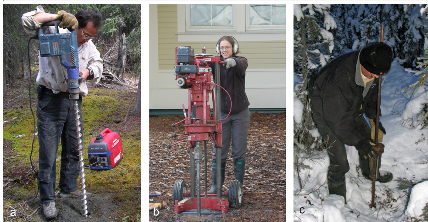
Figure 1. Portable apparatus used for drilling shallow boreholes: (a) electric hammer drill; (b) gasoline-powered Minuteman water jet drill; and (c) manual percussion drill.
