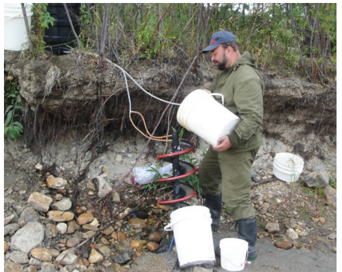
Figure 2. Dr. Vladimir Naumov operating a 'Screw Sluice' test plant on the banks of Indian River.
