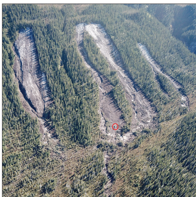
Figure 2. Active layer detachment slides at the confluence of Arch Creek and Donjek River. Helicopter (circled) for scale. The initiation zone is ~150 m vertically above the toe and the track is ~500 m long. These active layer detachment slides are quite large with respect to others seen in this region.
