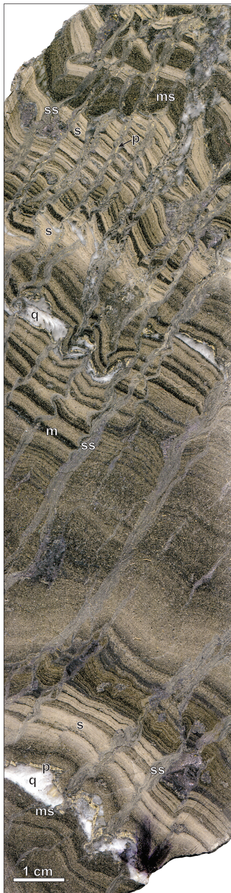
Figure 9. Drill core through a deformed section of the Active Member at the XYC deposit. Sulphide-rich and mudstone laminae are crosscut at a high angle by sulphide seams. The sulphide-rich laminae and the sulphide seams are largely made up of sphalerite and pyrite. Galena was rarely identified and is concentrated in the seams rather than the laminae. m = mudstone; ms = mudstone with disseminated sulphide; s = sulphide-rich laminae; p = pyrite; ss = sulphide seam; q = extensional quartz veinlets. Core is from XYC-235 at 86.70 m.
