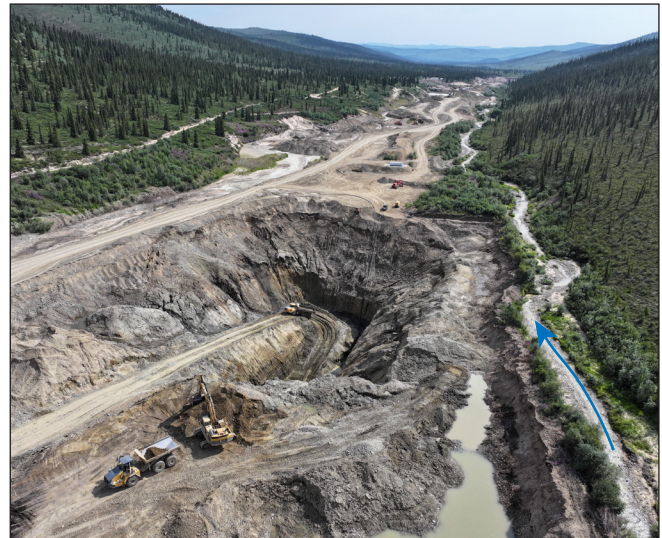
Figure 19. Rock Bottom Mining's 2024 activity on Nansen Creek, downstream from the mouth of Discovery Creek, where they were targeting a deeply buried paleochannel. The blue line shows stream flow direction. The view is downstream and to the south.
