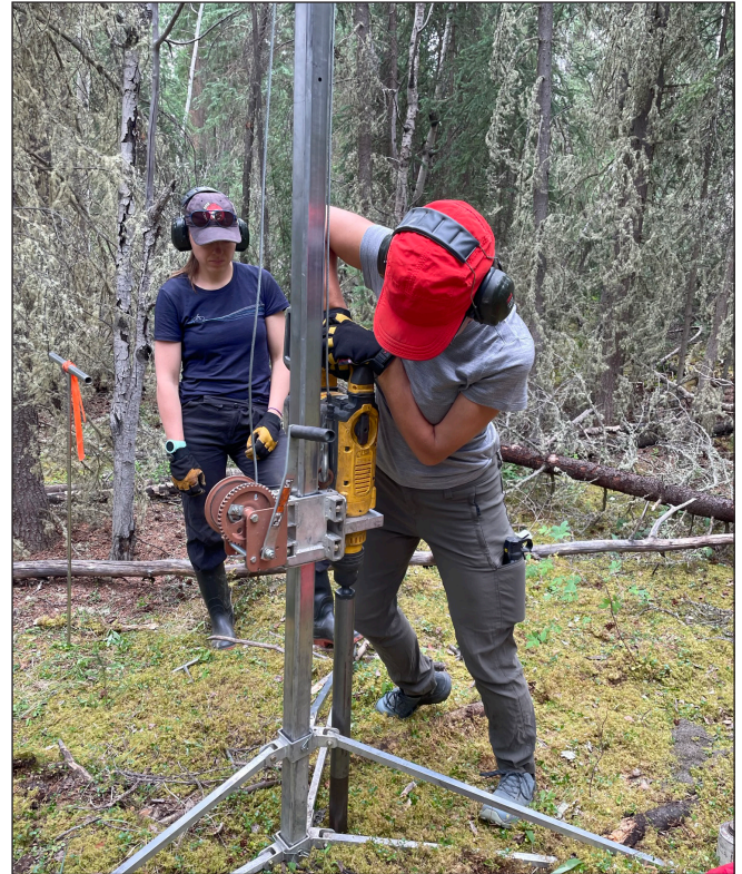
Figure 8. Moya Painter and Emilie Stewart-Jones drilling a borehole to monitor permafrost in Ross River.
