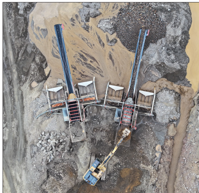
Figure 14. Drone image of a Caterpillar 349 excavator feeding two screen decks in tandem at H.C. Mining Ltd.'s upper Henderson Creek operation near the confluence with Cabin Creek.
