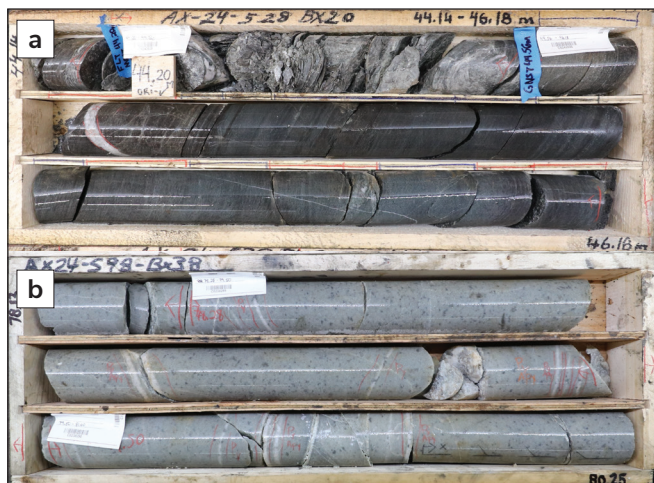
Figure 8. Core photos from drillholes. Core diameter is 71 mm (HTW). (a) Mafic sills/volcanic units in drillhole AX-24-528. (b) Aplite dike in drillhole AX-24-598.
