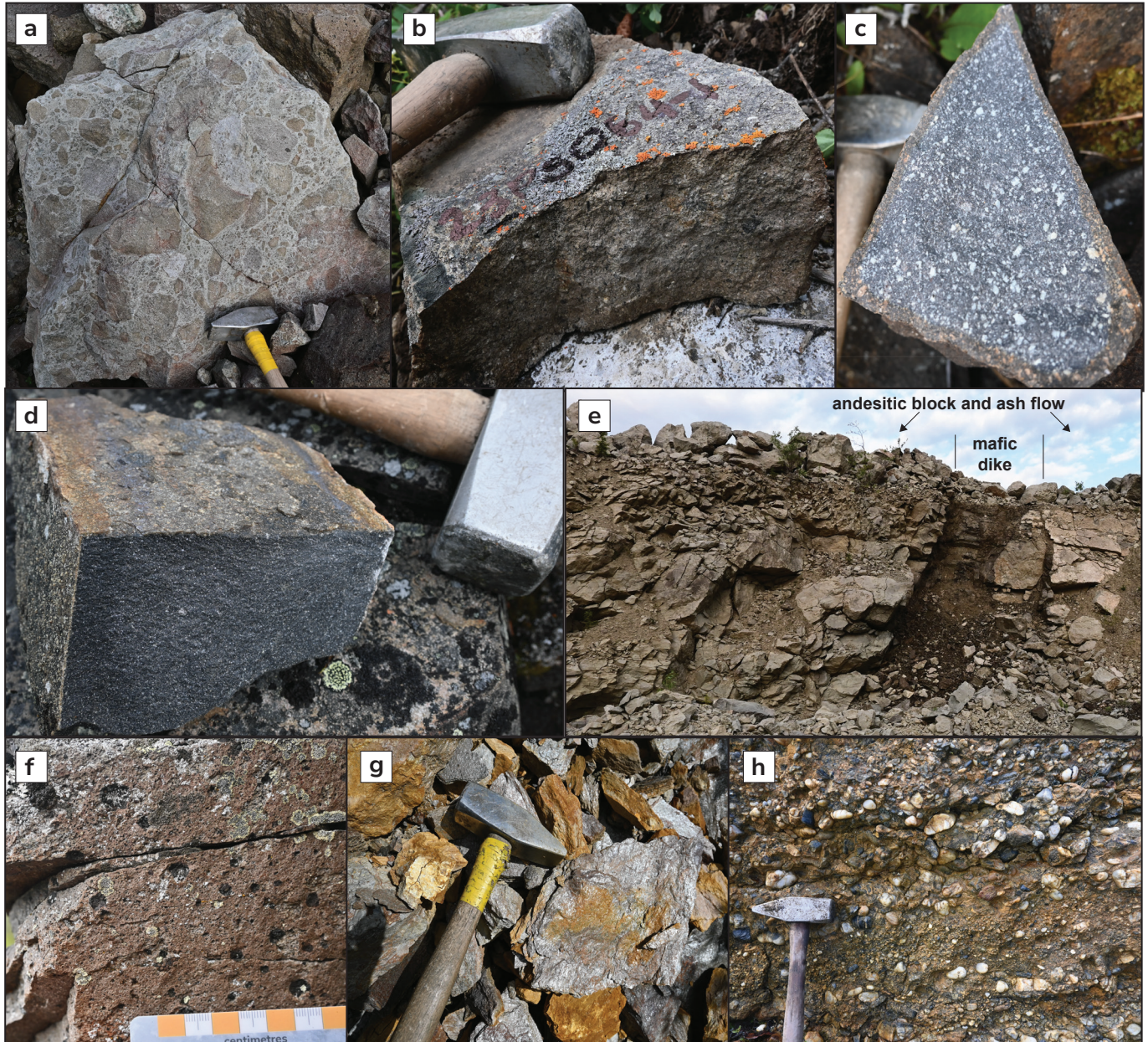
Figure 6. Field photographs of select outcrops and hand samples: (a) pyroclastic breccia; (b) crystal tuff; (c) massive plagioclase porphyritic andesite; (d) plagioclase porphyritic basaltic andesite; (e) mafic dike cross-cutting andesitic block and ash flow; quarry face is approximately 3 m high; (f) pyroxene porphyritic monzogabbro; (g) chlorite-muscovite-quartz schist; and (h) pebble conglomerate.
