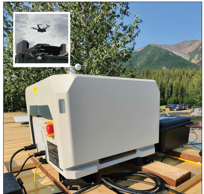
Figure 3. Installation of the DJI Dock 2 on the top of the shipping container; Miles Ridge is in the distance. The inset illustrates the M3TD during take-off. The Dock 2 weighs 34 kg and is 57 × 58.3 × 46.5 cm (L×W×H) with the doors closed.
