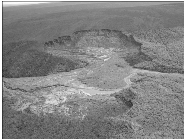
Figure 2.26: A “retrogressive thaw” in the Peel Watershed. An initial disturbance to the permafrost results in a slump, which in turn exposes more permafrost to thawing temperatures. The slump then expands away from the initial disturbance. Note the resulting disturbance to the creek. (Photo: D. Davidge, Environment Canada)
