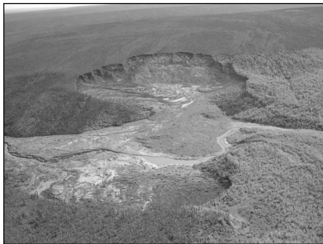
Figure 2.27: A “retrogressive thaw” in the Peel Watershed. An initial disturbance to the permafrost results in a slump, which in turn exposes more permafrost to thawing temperatures. The slump then expands away from the initial disturbance. Note the resulting disturbance to the creek. (Photo: D. Davidge, Environment Canada)
