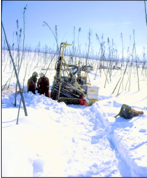
Figure 2.14: Winter exploration in Eagle Plains: setting up a portable drilling rig. (Photo: Yukon Energy, Mines, and Resources)
