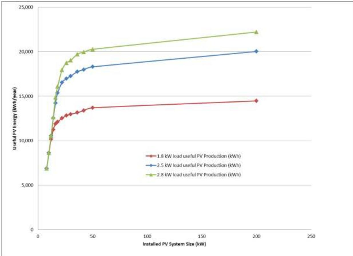
**Figure 7:** Useful energy from PV system vs. installed PV system capacity.
