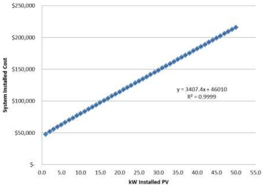
**Figure 6:** PV System installed Cost vs. PV System Capacity (kW).
