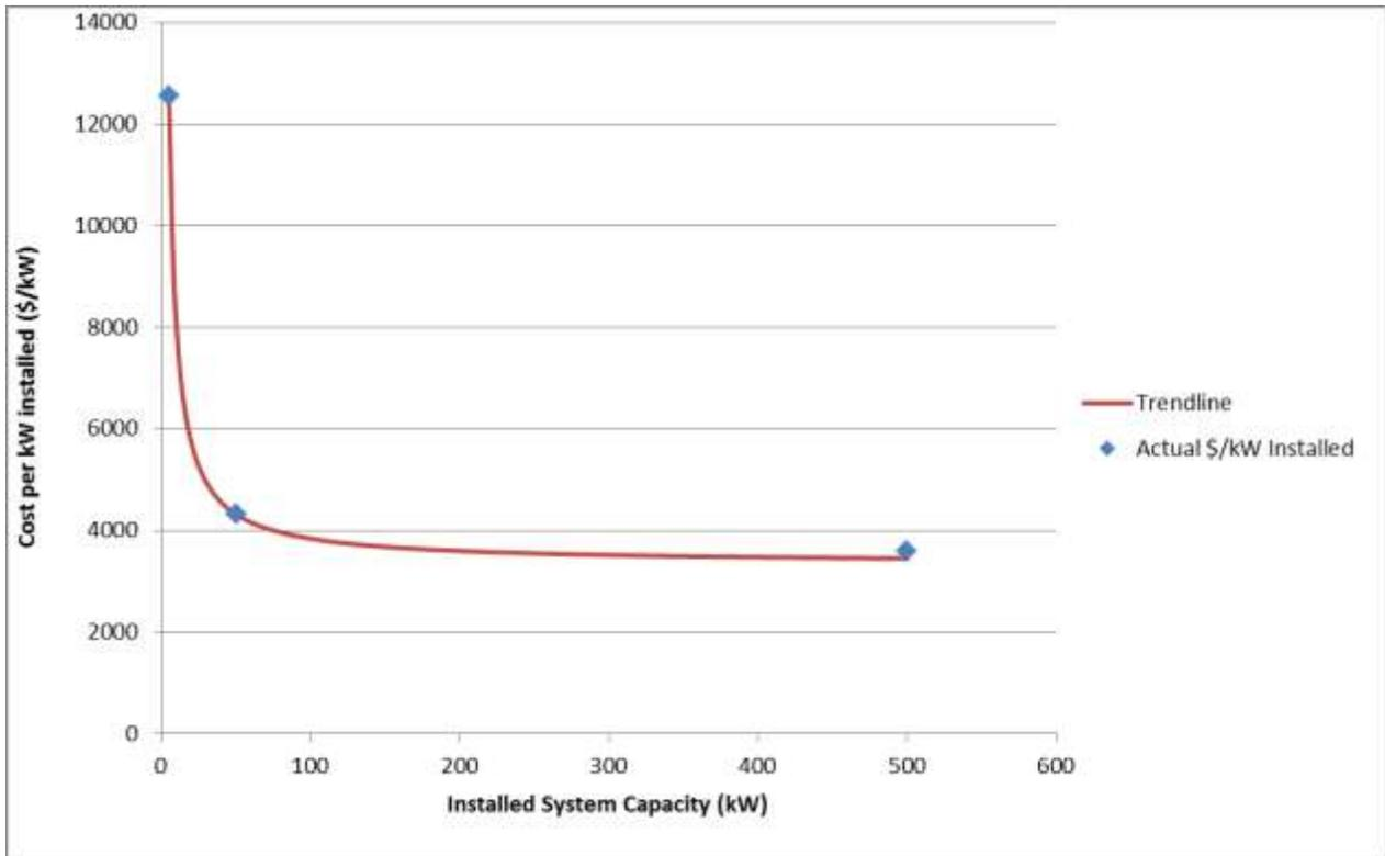
**Figure 5:** Relationship between installed PV system capacity-price (\$/kW installed) and installed PV system capacity.
