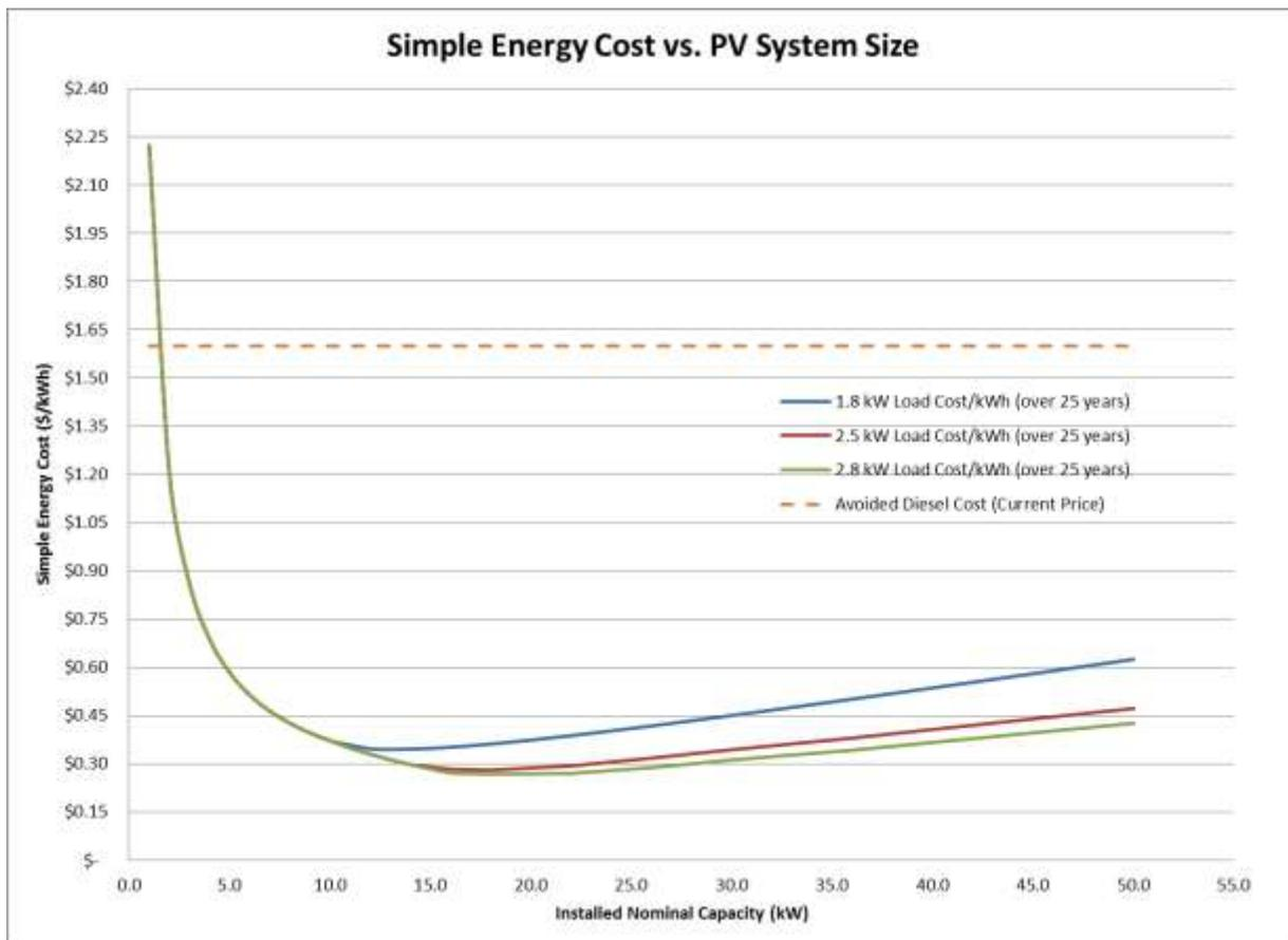
**Figure 8:** Simple PV Energy Price vs. Installed PV system Capacity (kW).
