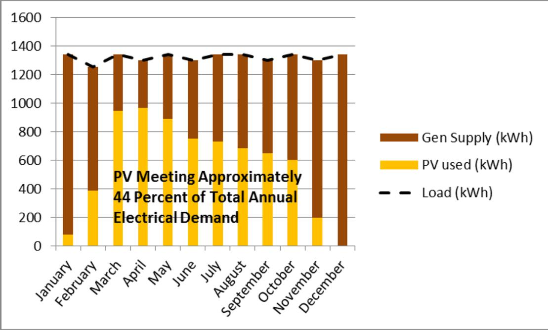
**Figure 2:** Simulation of an 8 kW solar PV system for a NWTel remote site with a constant 1.5 kW load.
