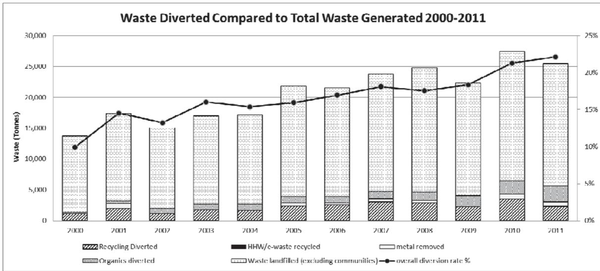
Note: Diverted metals include appliances, car bodies and other metals stockpiled that are shipped and processed south for recycling.
