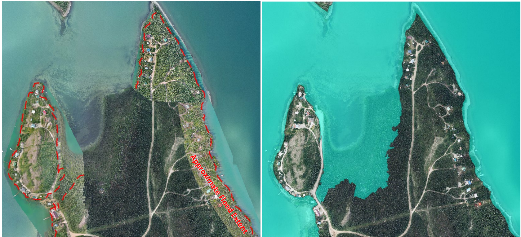
FIGURE 55: COMPARISON OF 2011 (LEFT) AND 0.5% AEP (RIGHT) FLOOD EXTENTS IN JACKFISH BAY
