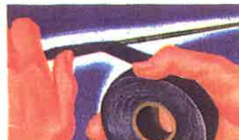
Rubber... Rubber Substitutes... Milled into rubber, Aroclors impart permanent tackiness and adhesion; also reduce brittleness.
