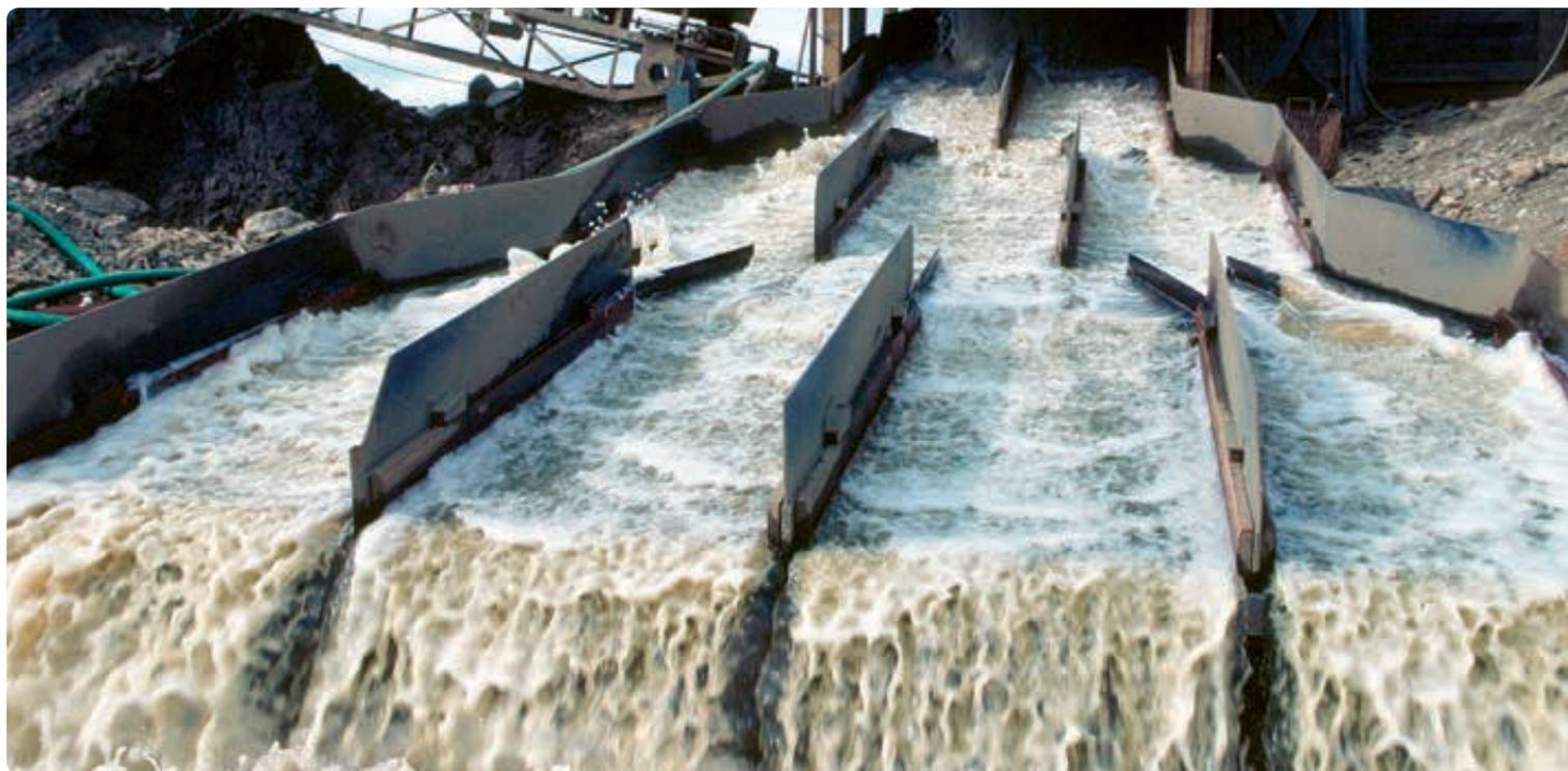
Placer mine sluice box in the Klondike region
