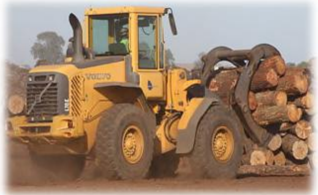
Wheel Loader with Log Grapple (Image courtesy Bob Adams, Flickr, CC BY-SA 2.0)
