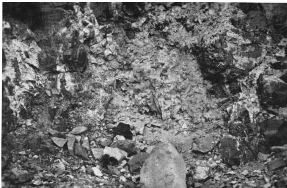
PLATE III. Dick vein-lode in cliff face showing brecciated basalt and fillings of calcite and quartz; a chalcocite content of 4 to 8 per cent is not visible in the photograph.
