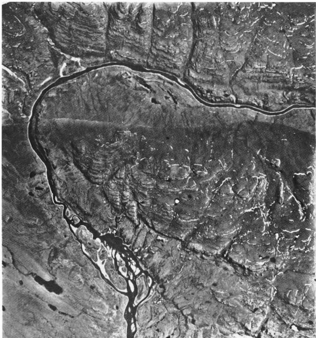
PLATE I. Coppermine Mountains (at top of photo) and September Mountains separated by Coppermine River; note fault and dyke lineaments and the terraces formed by north-dipping basalt flows.
