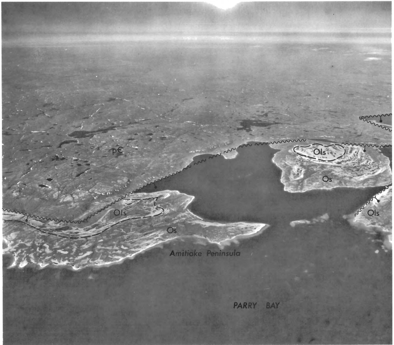
Plate 2. Fault zone west of Parry Bay; view to the west. (Symbols as on geological map). The Precambrian rocks form a plateau that probably represents the elevated, stripped, and somewhat eroded surface on which the lower Paleozoic succession was deposited. The vertical separation of the fault probably exceeds 1,000 feet (300 m). Oblique aerial photograph T-247-R-102
