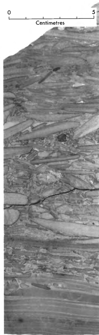
Plate 53. Dolomitic flat-pebble conglomerate, silty and very fine grained sandy, underlain by laminated dolostone; Ship Point Formation, member B, unit 149, 1306.1 to 1306.65 feet. PRA-033-22
