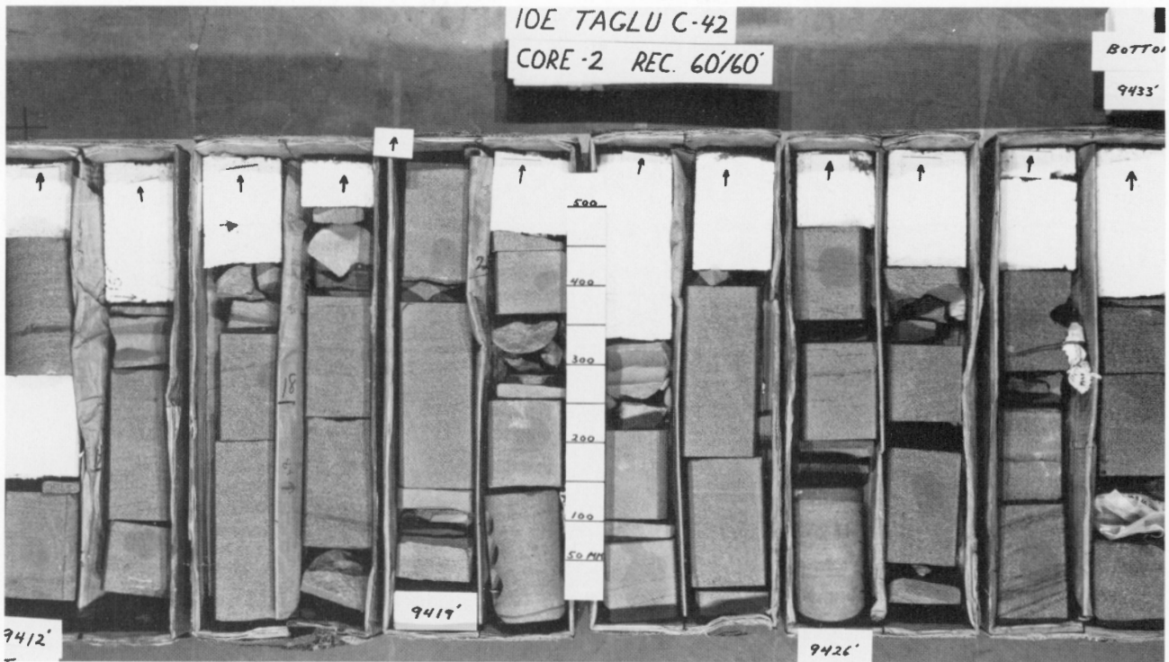
Figure 11. Slabbed core of typical sandstone of Reindeer Formation, Imperial Taglu C-42 well, Core no. 2, 2869-2875 m (9412-9433 ft). ISPG Photo No. 875-3.
