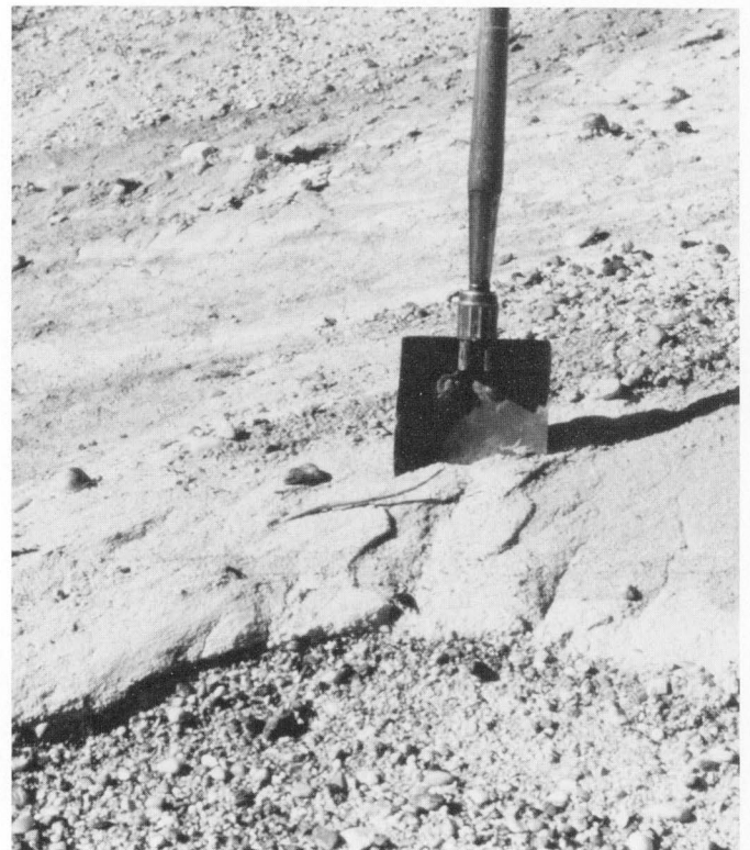
Figure 18. Friable sandstone and expandable, soft mudstone of the Kugmallit Formation; Imperial Netserk F-40 well; Core no. 1; 1853-1862 m (6078-6108 ft). ISPG Photo No. 910-10.
