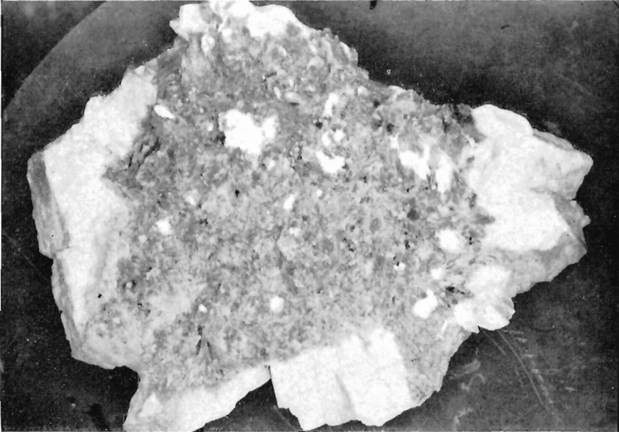
Late muscovite replacing quartz (extreme top and top left) and perthite along zone contact; hand specimen from dyke 84.
