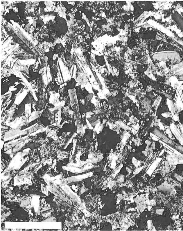
Figure 37. Photomicrograph of fresh quartz-bearing pigeonite diabase from post-Archean dyke cutting the Sunset Lake belt south of Payne Lake. Scale bar 2 mm long. GSC 190982
