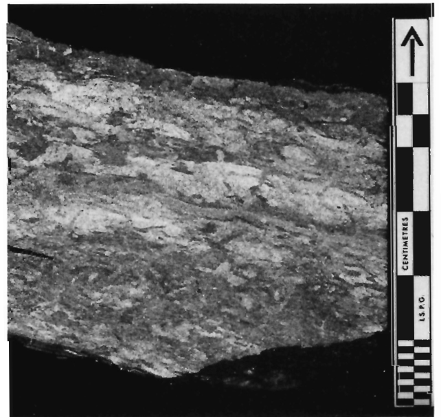
Figure 36. Bioturbated siltstone and sandstone of the Gaylard Member, near Peace River Canyon. ISPG photo. 2473-12.
