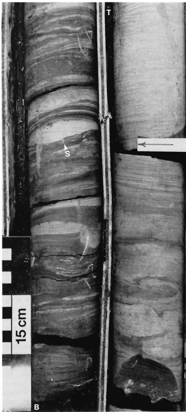
Figure 54. Close-up view of part of the core shown in Figure 53, illustrating syneresis crack (S), and distorted laminae in sandstone. Top of core (T). Bottom of core (B). ISPG photo. 2674-19.
