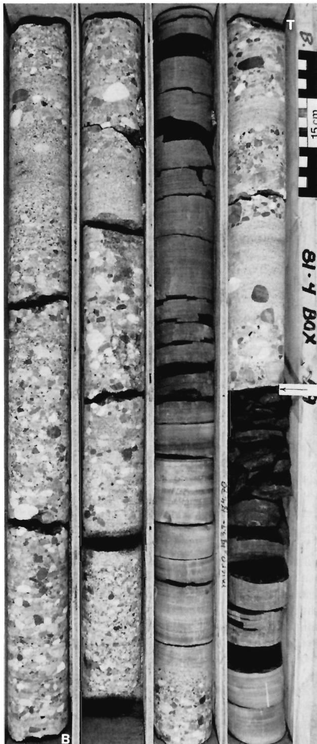
Figure 49. Conglomerate, conglomeratic sandstone, siltstone and mudstone of the Chamberlain Member, Monkman–Stony Lake area, in core from Petro-Canada DDH 81-04. Note fining-upward character of the conglomerate-sandstone, and sharp erosional base of the upper conglomeratic sandstone and conglomerate. Top of core (T). Bottom of core (B). ISPG photo. 2674-6.
