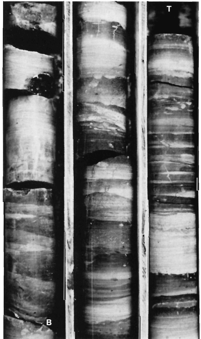
Figure 22. Rhythmic alternations of light weathering, very fine grained sandstone to siltstone and darker weathering mudstone in core from the upper Gaylard Member at borehole BP 53. Note fining-upward, sharp based sandstone tempestites or turbidites, well developed syneresis cracks, and horizontal Planolites -like burrow traces. Top of core (T). Bottom of core (B). ISPG photo. 2470-2.
